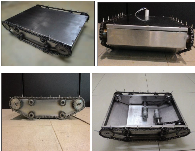
Figure 5. The prototype of ROC inside view.
