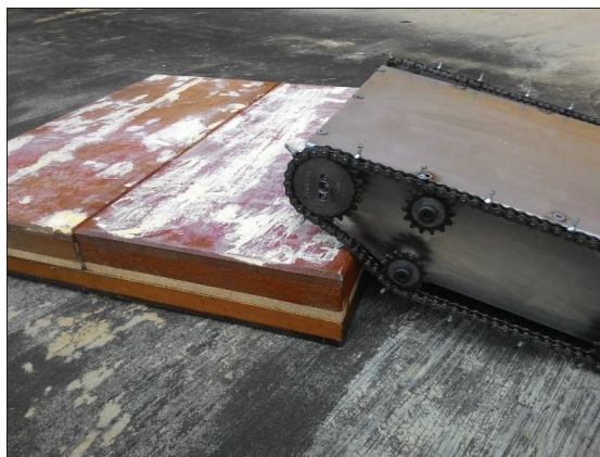
Figure 12. The crawler climbed the 9.5 cm obstacles.
