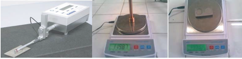
Figure 3. Digital surface roughness tester and electronic balance used
