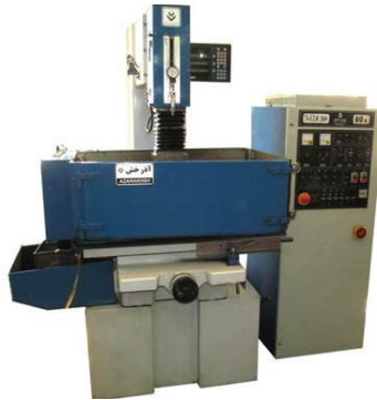
Figure 3. The Azerakhsh-304H EDM machine used for experiments
