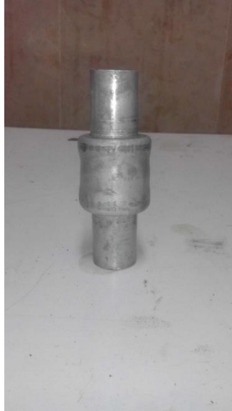
Figure 5. The hydroformed stepped tube with the proposed die and mechanism
