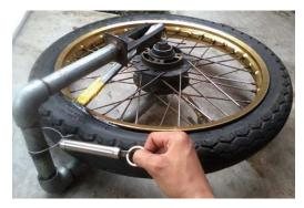
FIGURE 9 Measuring the required force to pull or push the tool handle
