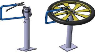
FIGURE 8 Final concept of the motorcycle tire dismounting tool
