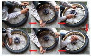
FIGURE 2 Current practice of the motorcycle tire dismounting process
