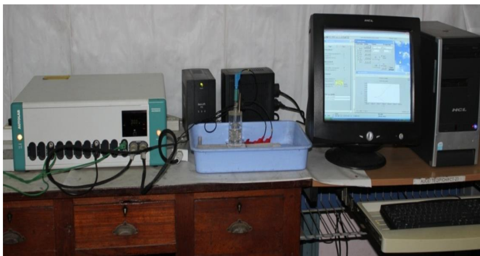
Figure 4. Pitting corrosion setup
