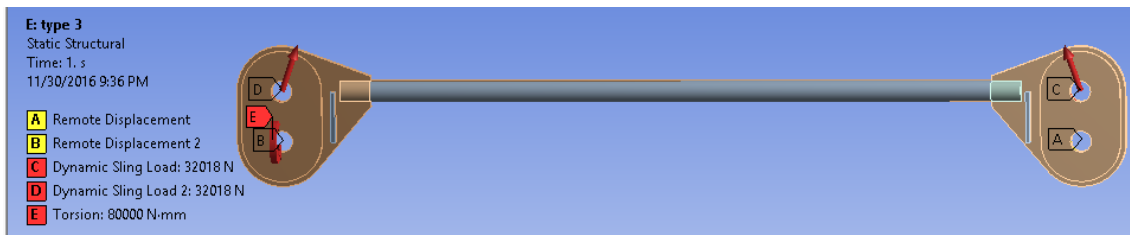
Figure 10 (a). Loading and boundary condition applied to the SB type 3
