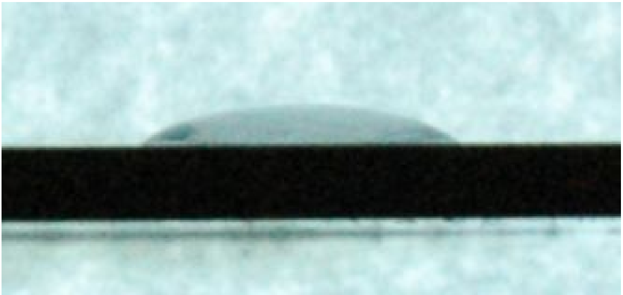
Figure 3.14. 50 \mu L of a 0.1% surfactant mixture placed on a polished aluminum surface.
