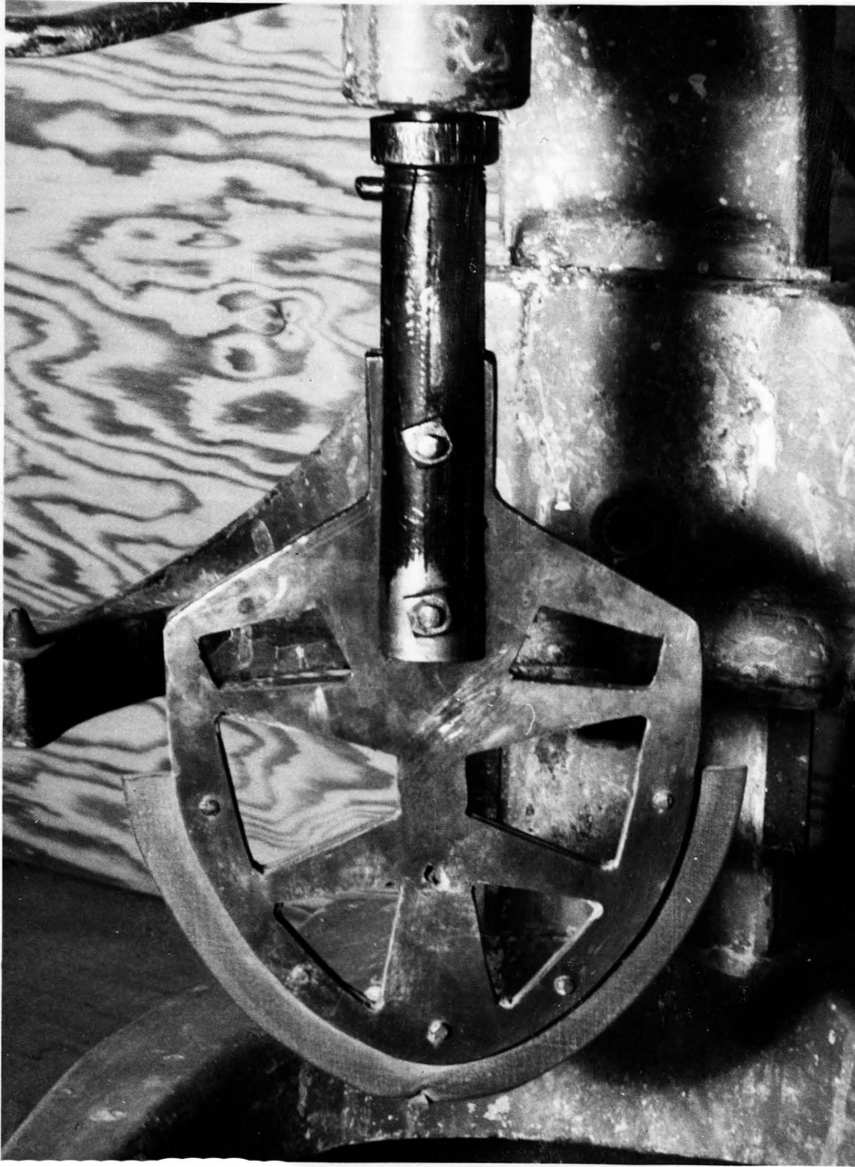
Figure 3. Mixer Blade, showing details of construction. Rubber scraper around lower part of blade is clearly shown. Stem was made from a length of pipe, slotted to receive blade.
