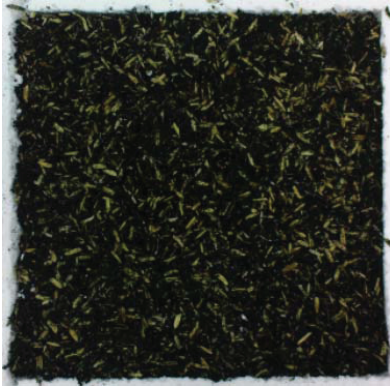
Figure 3: Rice husks-rubber tire dust particle board
