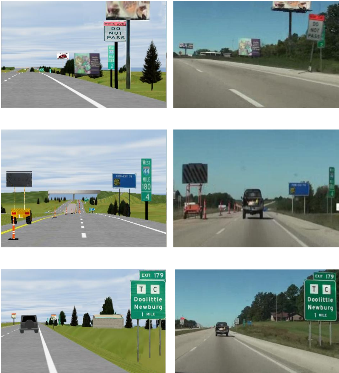
Figure 2. Comparison of Driving Simulator Scenarios (left) and Real World Captured Using a Video Camera (right)
