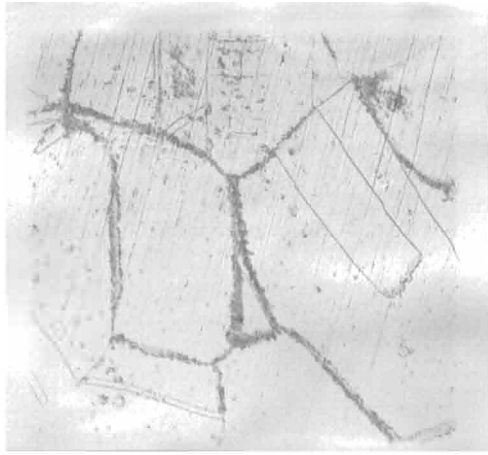
Figure 16 500X Alloy 11-60% Cu 40% MnNi
