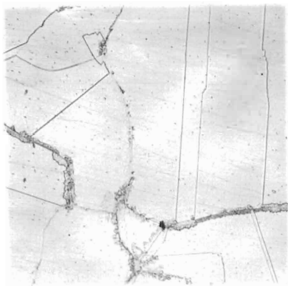
Figure 7 100X 60/20/20 1650°F-2hrs.-WQ Aged 750°F-24hrs.-WQ Dichromate Etch
