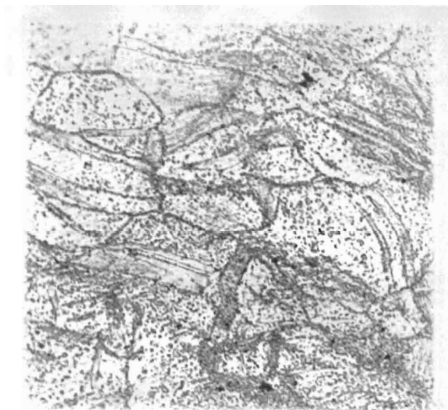
Figure 12 500X 60/20/20 1300°F-3hrs.-WQ Swaged-Aged 825°F-24hrs.-WQ Dichromate Etch
