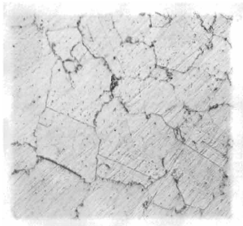
Figure 15 500X Alloy 8-70% Cu 30% MnNi
