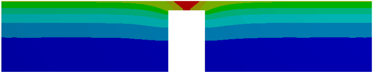
Figure.4.3 Lock-in Thermography on wide defect
