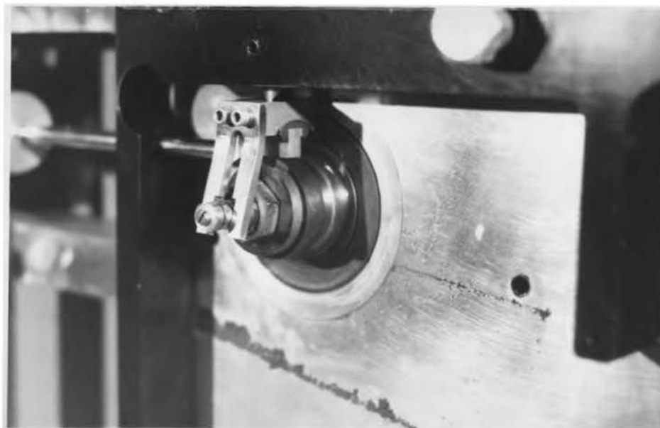
Fig. 5 Close-Up View of Ring and Block Assembly on LFW-1 Machine
