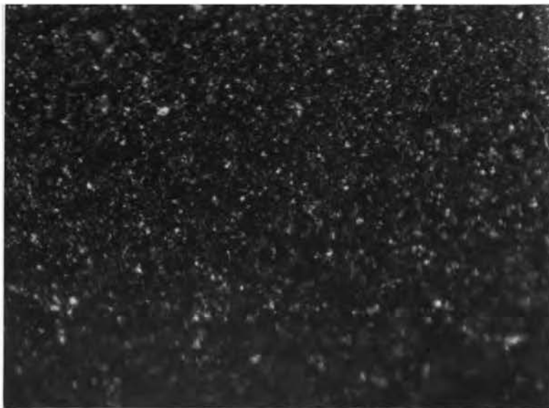
Fig. 21 Ring Surface after Coated with Solid Film Lubricant at 100X
