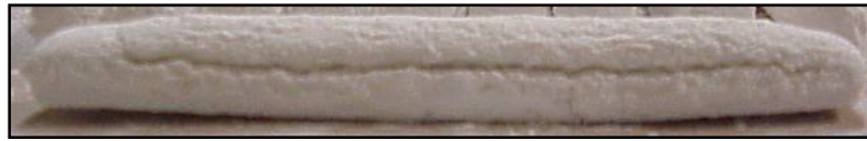
Figure 4.4: Example of severe surface cracking of green part
