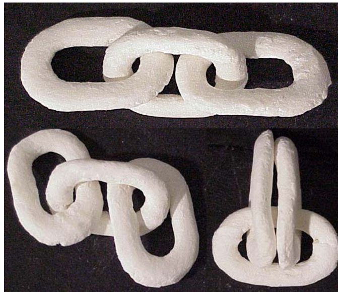
Figure 4.22: Alumina chain links produced by SLS
