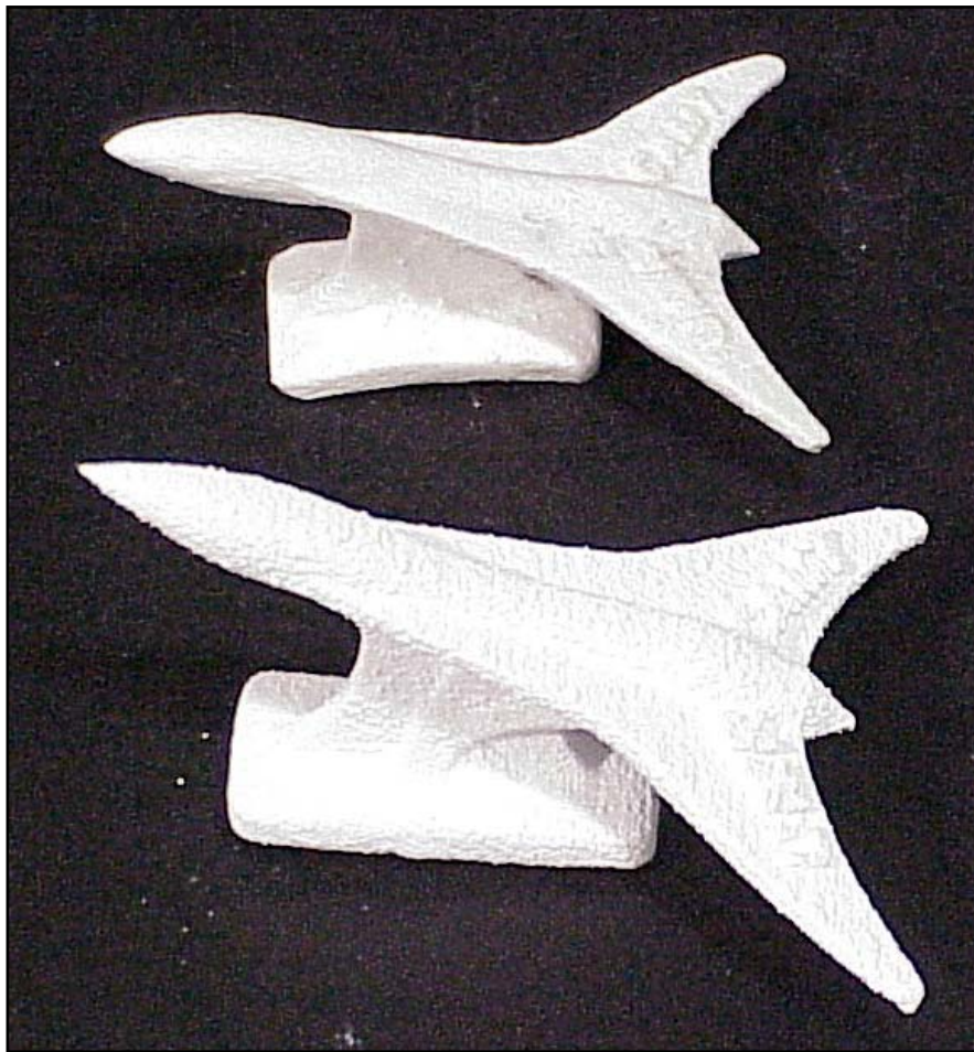
Figure 4.21: Green plane (bottom) and fully sintered plane (top)
