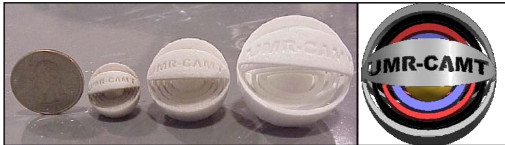
Figure 1.6: SLS parts – 5 independent, free-spinning balls in one made at UMR
