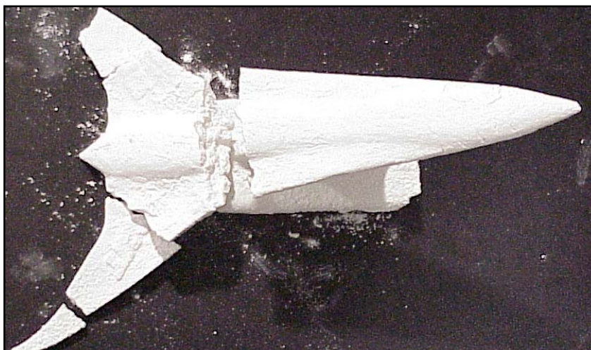
Figure 4.20: Plane broken during binder burnout
