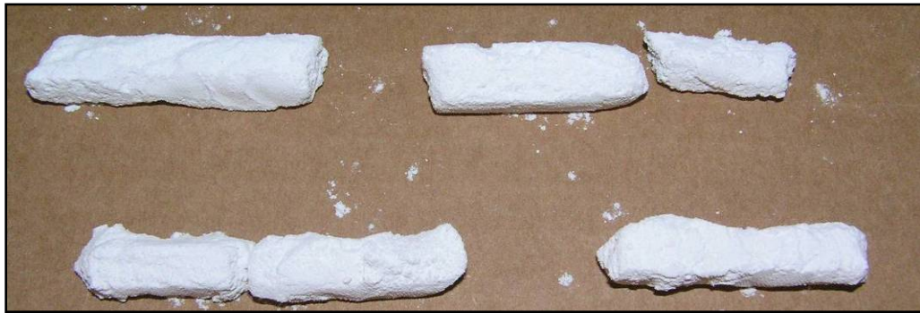
Figure 4.2: The best results achieved in this research using PMMA as a binder
