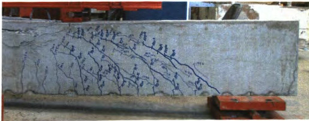
Figure 6.50. Control-5-2 Beam at Failure
