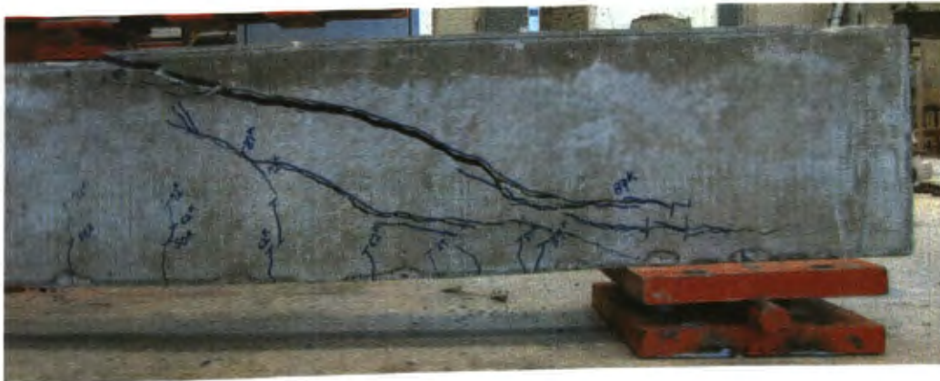
Figure 6.45. Control-NS-3 Beam at Failure
