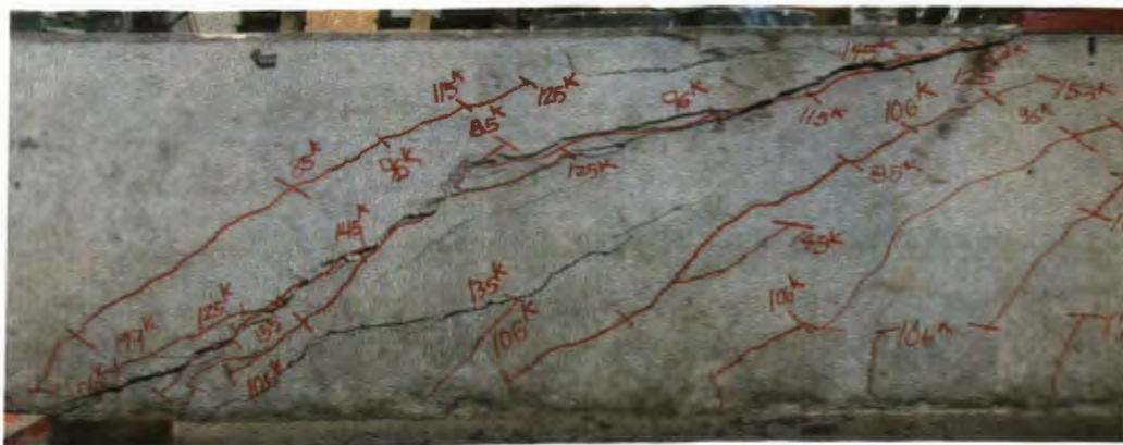
Figure 6.48. Control-7-3 Beam at Failure
