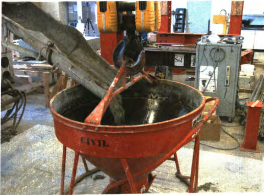
Figure 6.10. Filling Concrete Bucket
