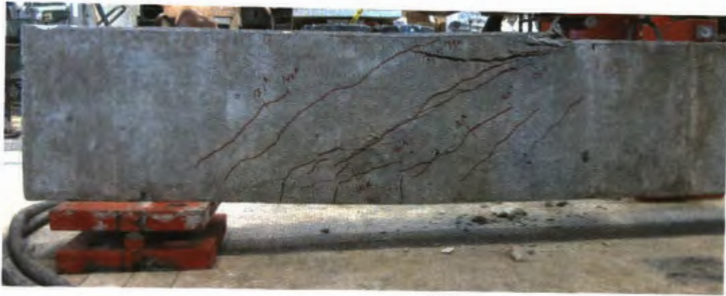
Figure 6.46. Control-7-1 Beam at Failure
