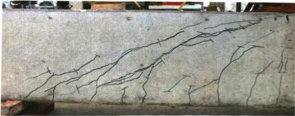
Figure 6.47. Control-7-2 Beam at Failure
