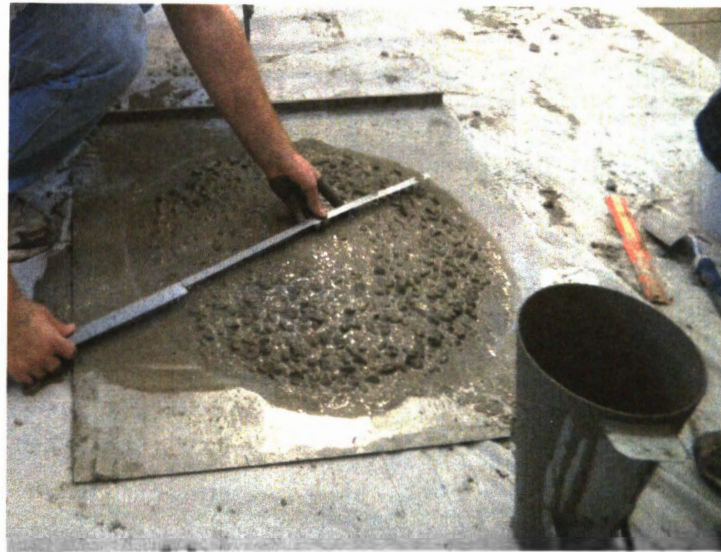
Figure 4.2. Measure Concrete Diameter During Slump Flow Test
