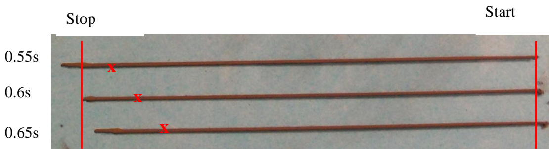
Figure 23 : Stop time tests for trajectory Method Conducted with Zirconium Diboride paste at Times of 0.55 s, 0.6 s and 0.65 s. Extrusion force 150 N. Table Velocity 5.3 mm/s. Standoff Distance is 55% of Extrudate Diameter. 'x' Controller Off.
