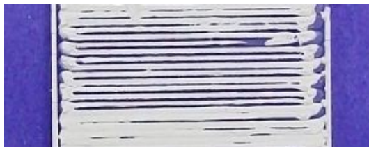
Figure 33 (continued): Rastering Conducted with Alumina and Overlap Factors of (a) -30%, (b) -35%, (c) -40%, (d) -45%, (e) -50%, (f) -55%, and (g) -60% .Standoff distance is 55%.Extusion force is 450 N. Table velocity is 4.868 mm/s. EOD Dwell Method is used.
