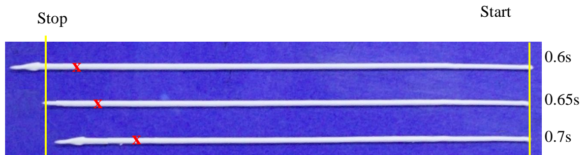
Figure 21: Stop Time Tests for Trajectory Method Conducted with Alumina Paste at Times of 0.7 s, 0.65 s and 0.6 s. Extrusion Force is 450 N. Table Velocity is 4.9 mm/s. Standoff Distance is 55% of Extrudate Diameter. 'x' Controller Off.
