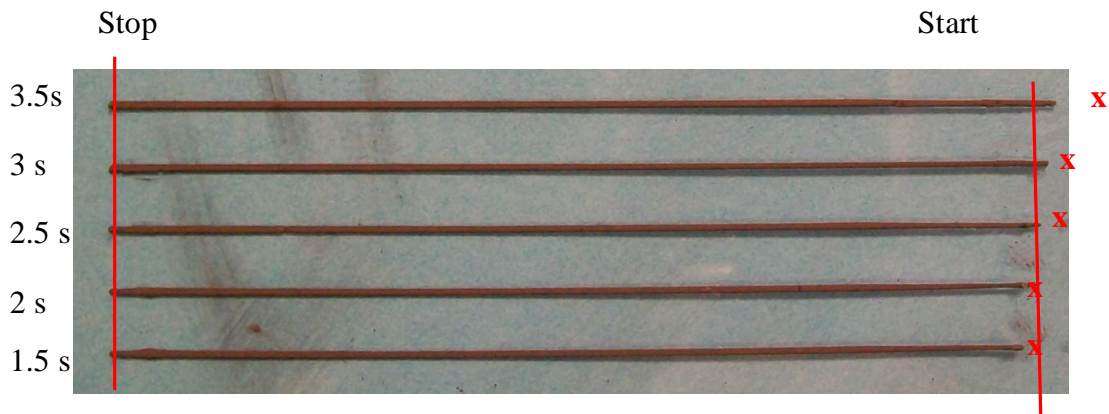
Figure 22: Start Time Tests for Trajectory Method Conducted with Zirconium Diboride Paste at Times of (a) 3.5 s, (b) 3.0 s, (c) 2.5 s, (d) 2.0 s and (e) 1.5 s. Standoff Distance is 55%. Extrusion Force is 150 N. Table Velocity is 5.3 mm/s. EOD Trajectory Method. 'x' Controller On.
