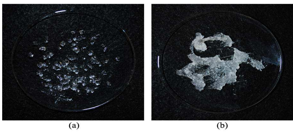
Figure 3-24. Comparison between initial and extruded 5.0 wt. % NaCl through 0.25 mm screen plate (a) initial (b) after extrusion.
