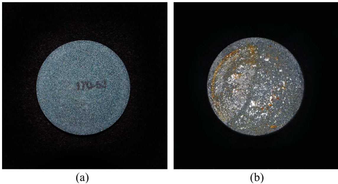
Figure 5-8. Comparison between initial surface of the ceramic disk and after filtration test for 2500 ppm viscous gel. (a) initial (b) after filtration test.
