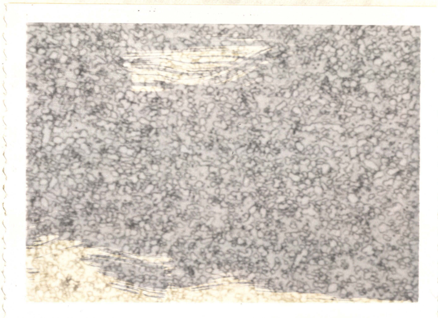
Fig. 8a: Two-Cycle Sample of A2 Steel. Sample No. A2-22. Sample held 1 hr at 1800°F, 2 hr at 1425°F, 1 hr at 1800°F, 2 hr at 1425°F, air cooled and then reheated 6 hr at 1425°F. 17 RC.
