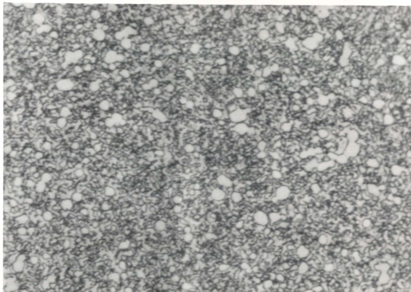
Fig. 5a: Mill Sample of M2 Steel. Sample No. M2-00. M2 steel as annealed in a tool steel mill. 18 RC.
