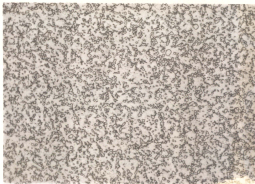
Fig. 8c: One-Cycle Sample of H13 Steel. Sample No. H13-21. Sample held 1 hr at 1800°F, 2 hr at 1525°F, air cooled and then reheated 6 hr at 1525°F. 8.5 RC.
