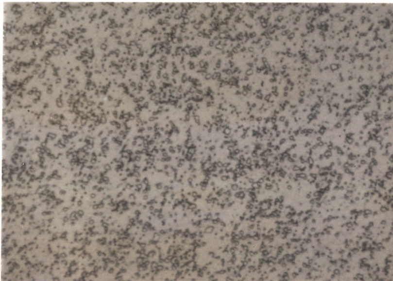
Fig. 12b: Hardened and Tempered Sample of H13 Steel. Sample No. H13-76. Sample heated at 1600°F for 1 hr and oil quenched. It was then tempered for 8 hr at 1525°F and furnace cooled. 9.5 RC.
