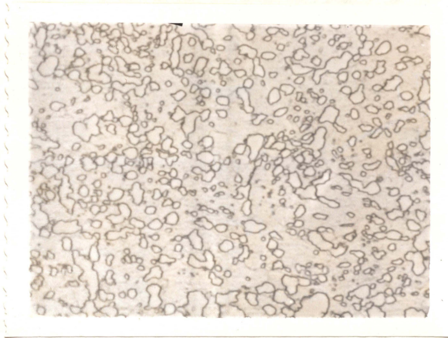
Fig. 13: Hardened and Tempered Sample of W1 Steel. Sample No. W1-74. Sample heated at 1500°F for 1 hr and oil quenched. It was then tempered for 8 hr at 1325°F and furnace cooled. 83 RB.
