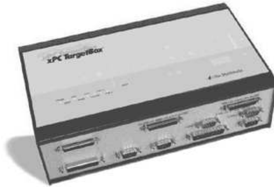
Figure 2.1. Mobile Mathworks xPC Targetbox® (270mm x 162mm x 82mm).
