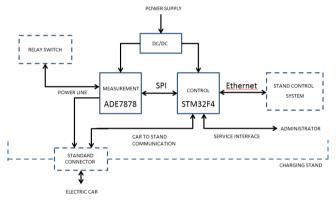
Figure 2: Proposed new architecture of charging stand
