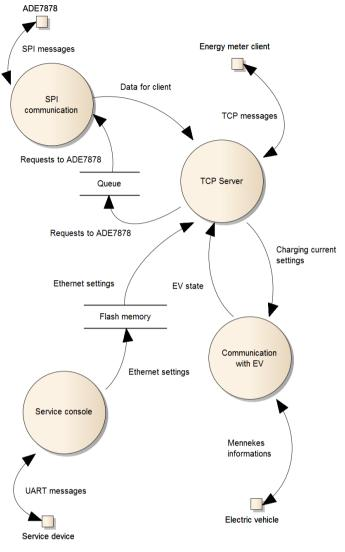
Figure 4: Data flow diagram of application
