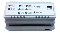
Figure 7: Energy meter developed for smart transportation purposes
