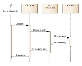
Figure 5: Sequence diagram of communication
