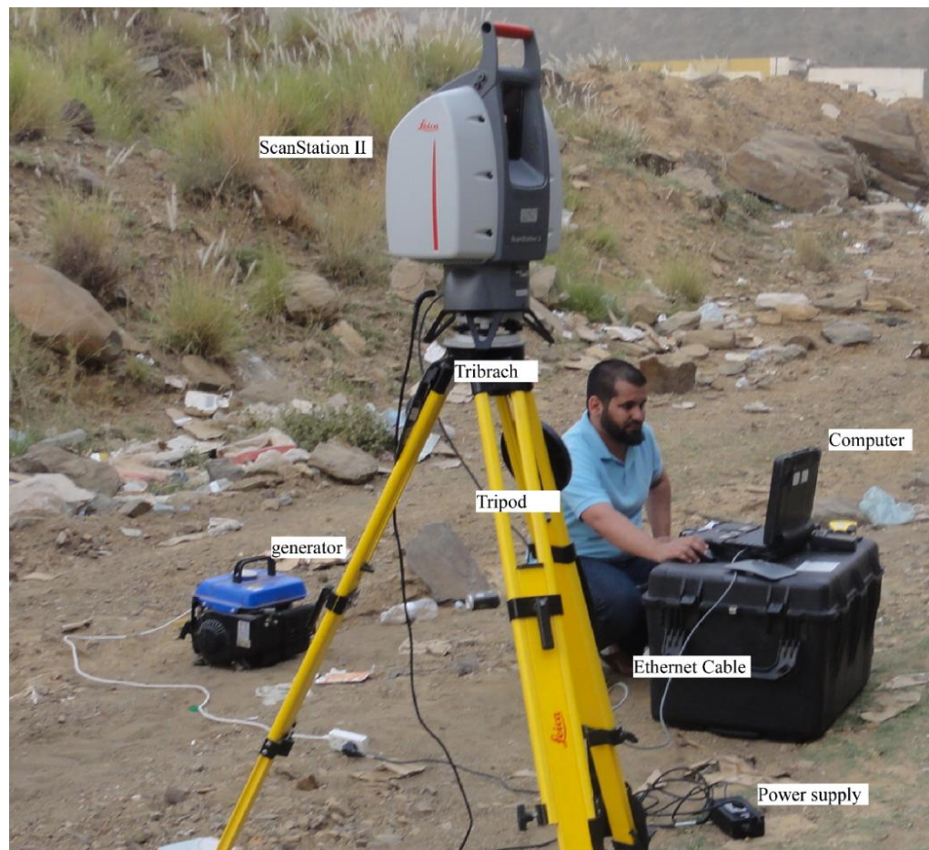
Figure 3.5. The picture shows the equipment used in collecting data
