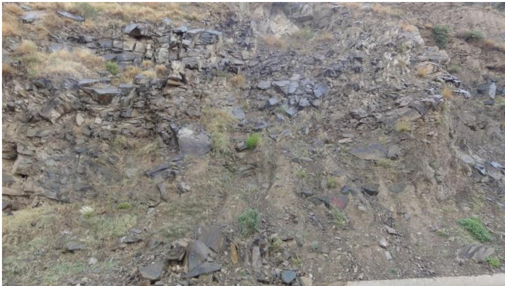
Figure 5.3. The picture shows Site A2, where sharp edge, disintegrated blocks of Basalt dominating the location
