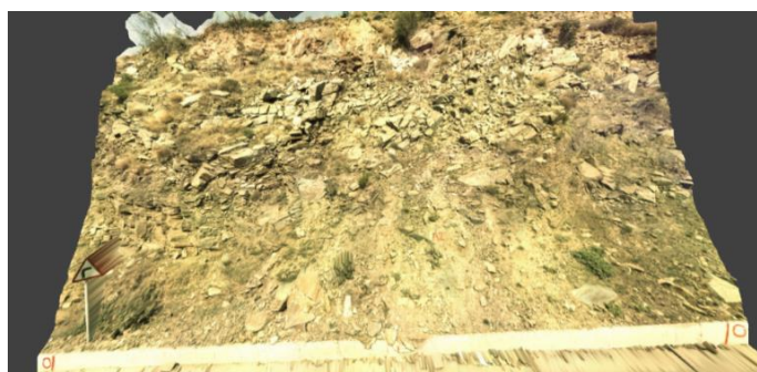
Figure 3.8. RGB image created from site A2 using ScanStation 2
