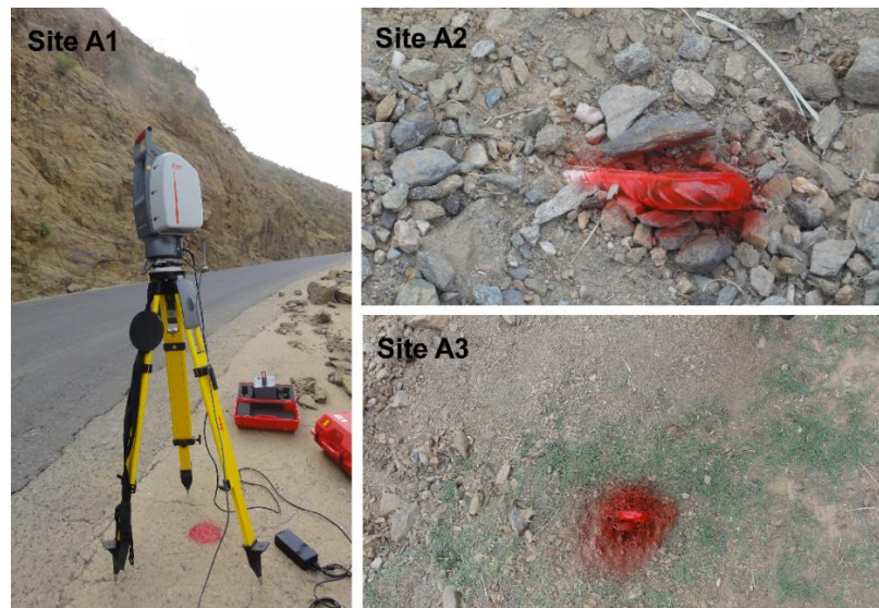
Figure 3.6. Fixed locations assigned for LiDAR ScanStation II for repeat scanning
