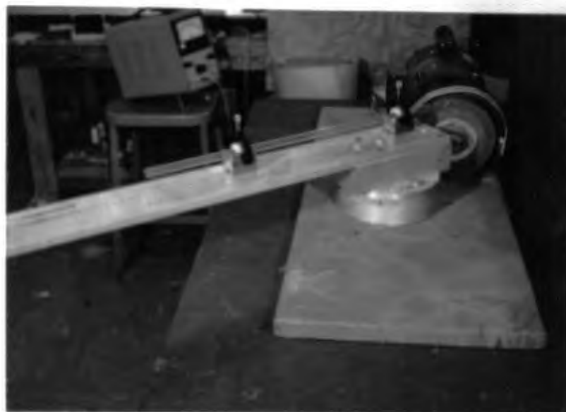
Figure 5. Window grinding method showing platform and Pyrex tube in mounting blocks
