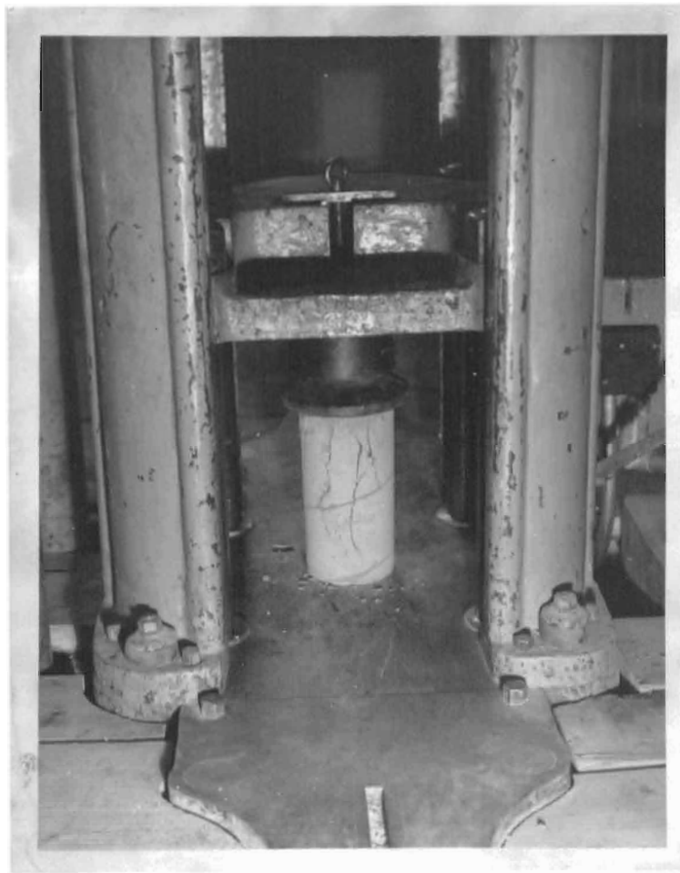
Figure 8. A Compression Test Cylinder a Few Seconds Prior to Reaching its Ultimate load.
