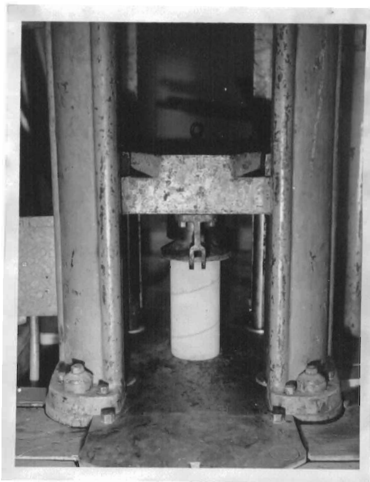
Figure 2. A Compression Cylinder that is About to be Tested to Failure in the 200,000# Tinius-Olsen Universal Testing Machine.
