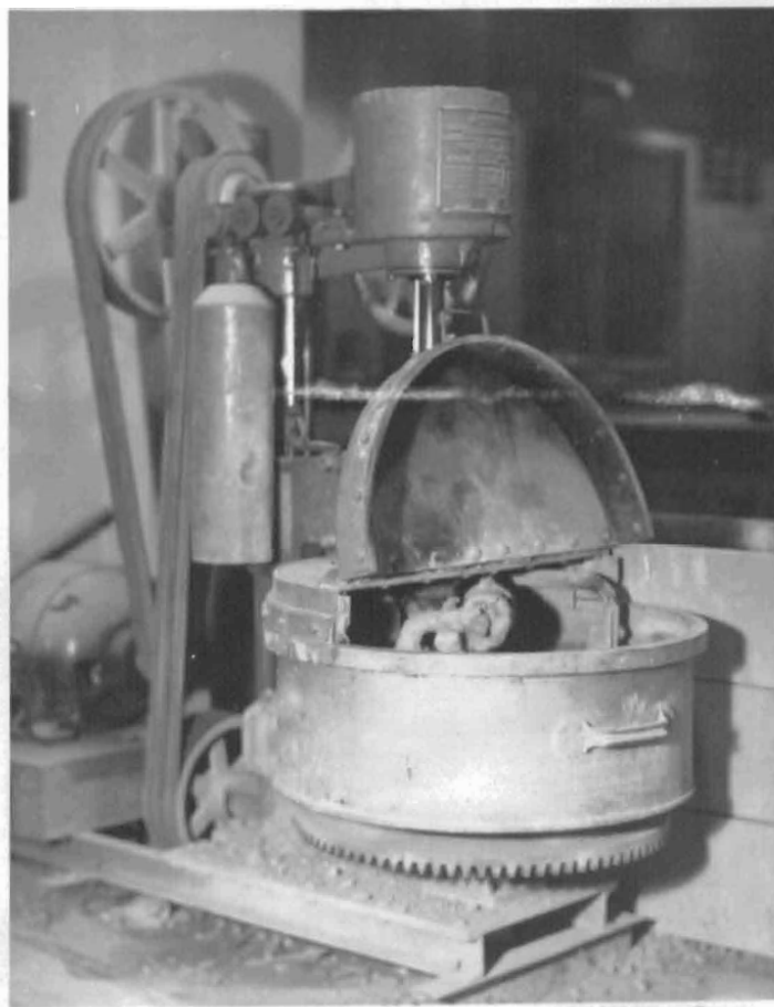
Figure 1. Lancaster Batch Mixer.
