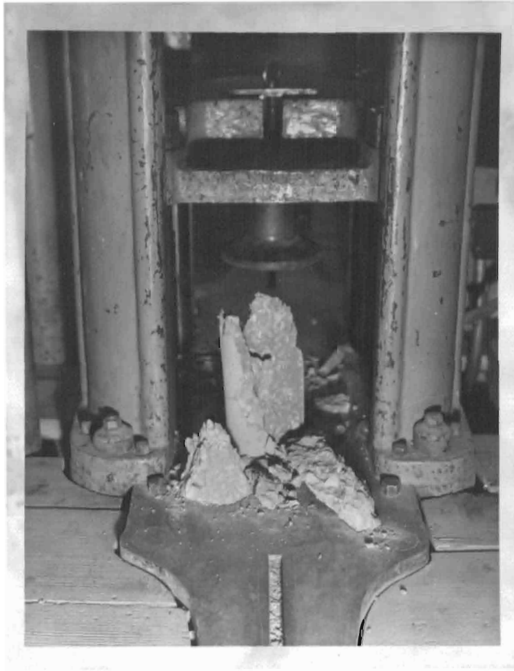
Figure 9. A Typical Failure of a Compression Cylinder for this Thesis Problem.
