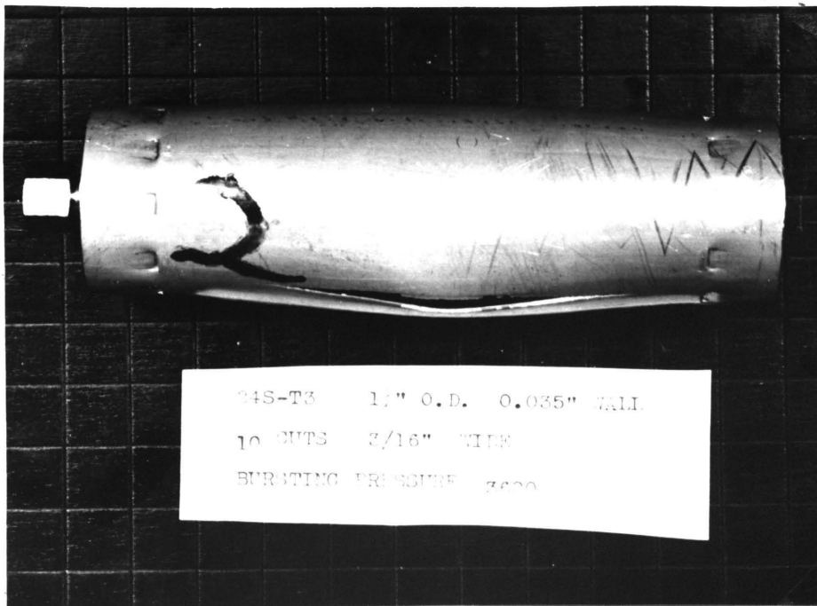
Figure 15. Photograph of the partial cut method, before and after failure.
