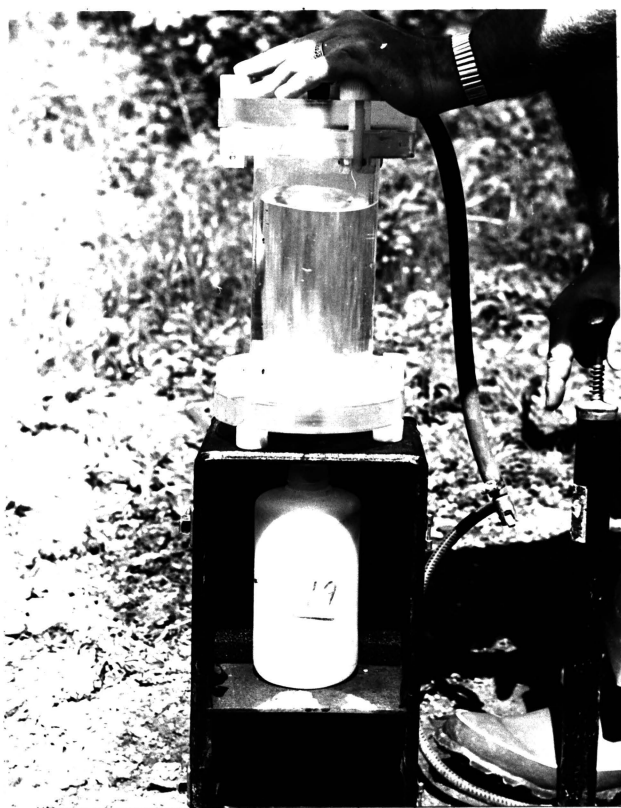
Figure 5: Field filtration of sample using the Skougstad filter assembly.
