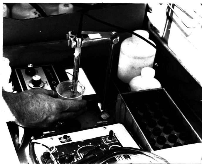
Figure 7: Field measurement - pH of unfiltered sample.
