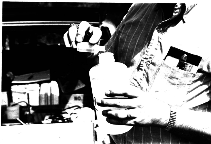
Figure 6: Sample acidification for retention of dissolved metals until analysis.
