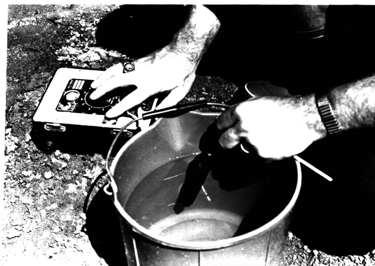
Figure 9: Field measurement - specific conductance of unfiltered sample.
