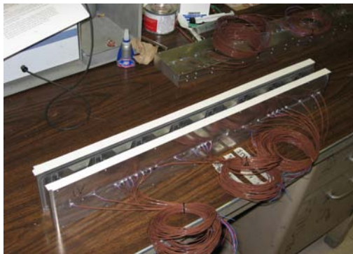
Figure 3.20: Ceramic paper glued to top of sides
