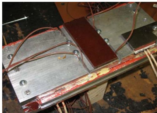
Figure 3.15: Phenolic piece positioned on heater
