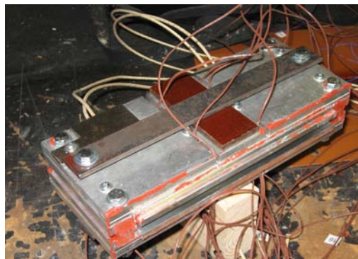
Figure 3.17: Heaters completely bolted to test section
