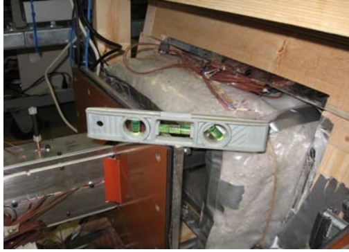
Figure 3.35: Leveling phenolic flange to match aluminum flange
