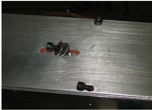
Figure 3.27: Bolts used to hold heaters in place
