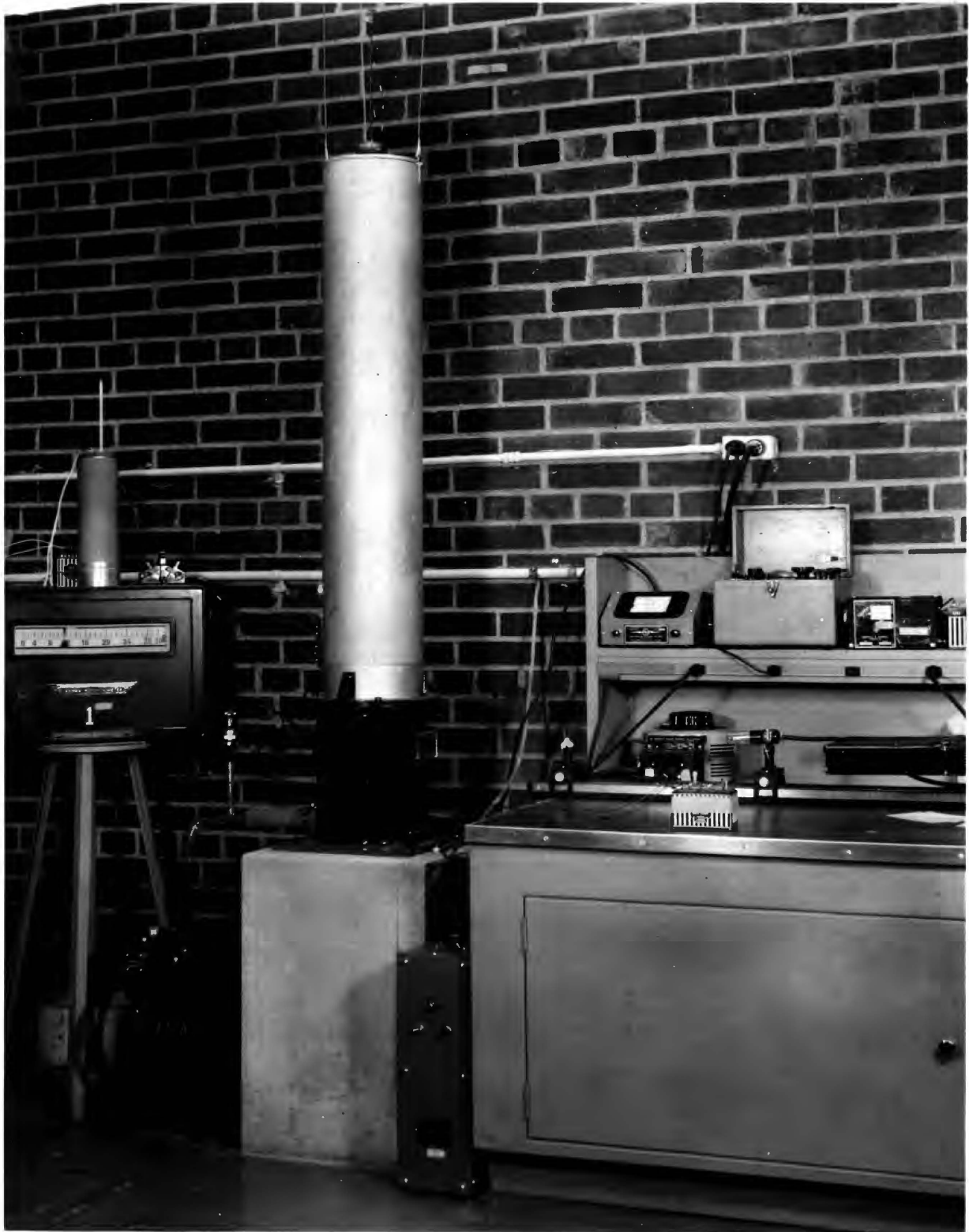
Arrangement of Ke Pendulum Apparatus (Photograph, courtesy of U. S. Bureau of Mines)
