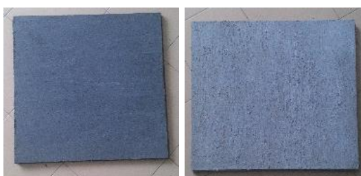
Figure 4: Plywood applied with (a) carbon (b) palm ash
