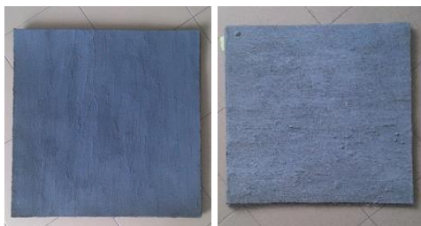
Figure 3: Board applied with (a) carbon (b) palm ash
