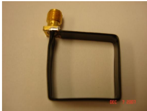
Figure 4.2. Copper Strap Wrapped in Electrical Tape
