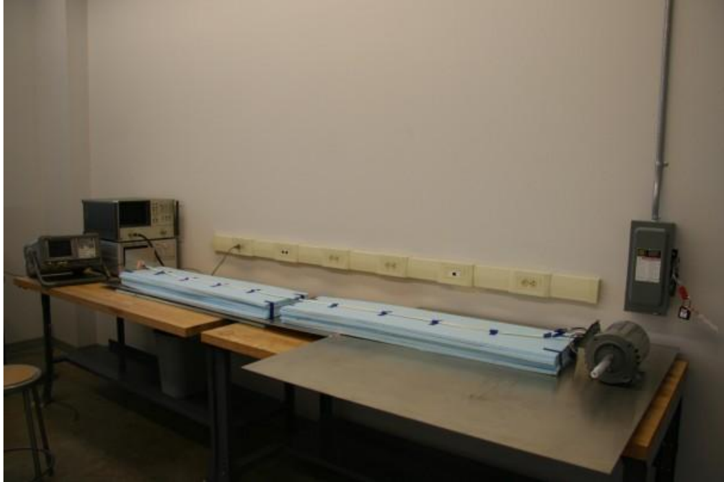
Figure 23 - Motor and Cable Test Setup: Full View
