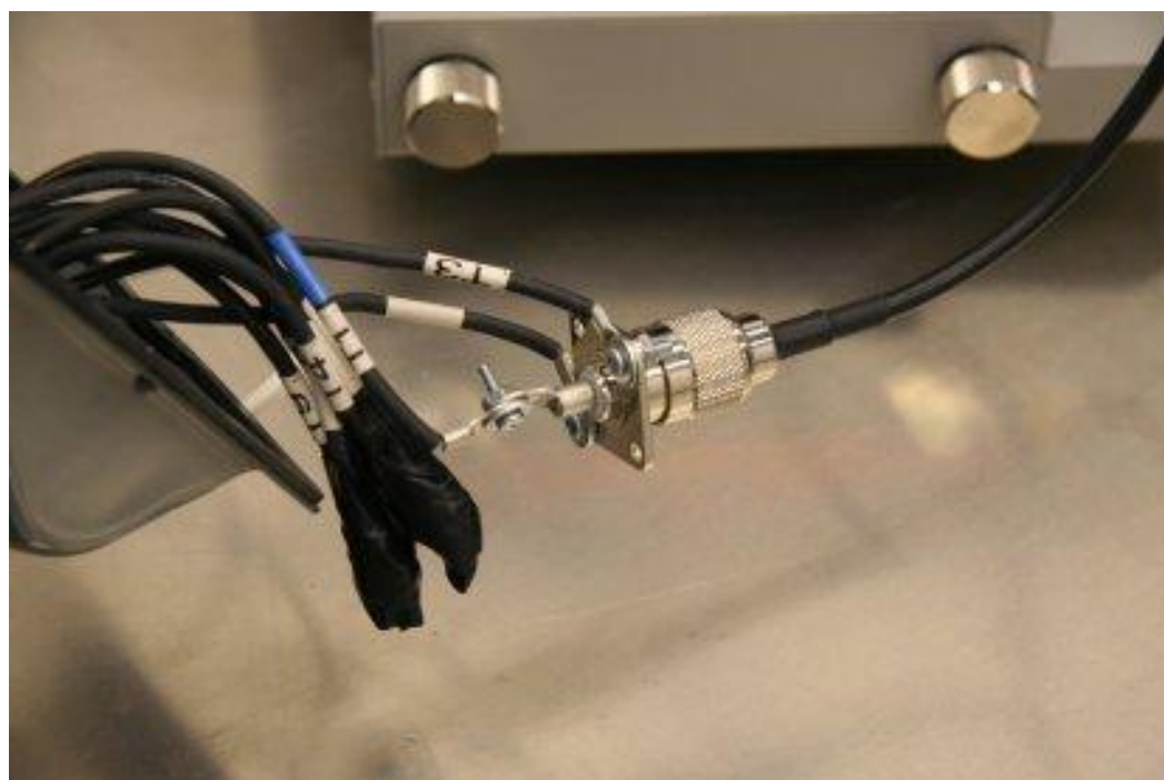
Figure 55 - Differential Mode Setup: Differential Mode Connection
