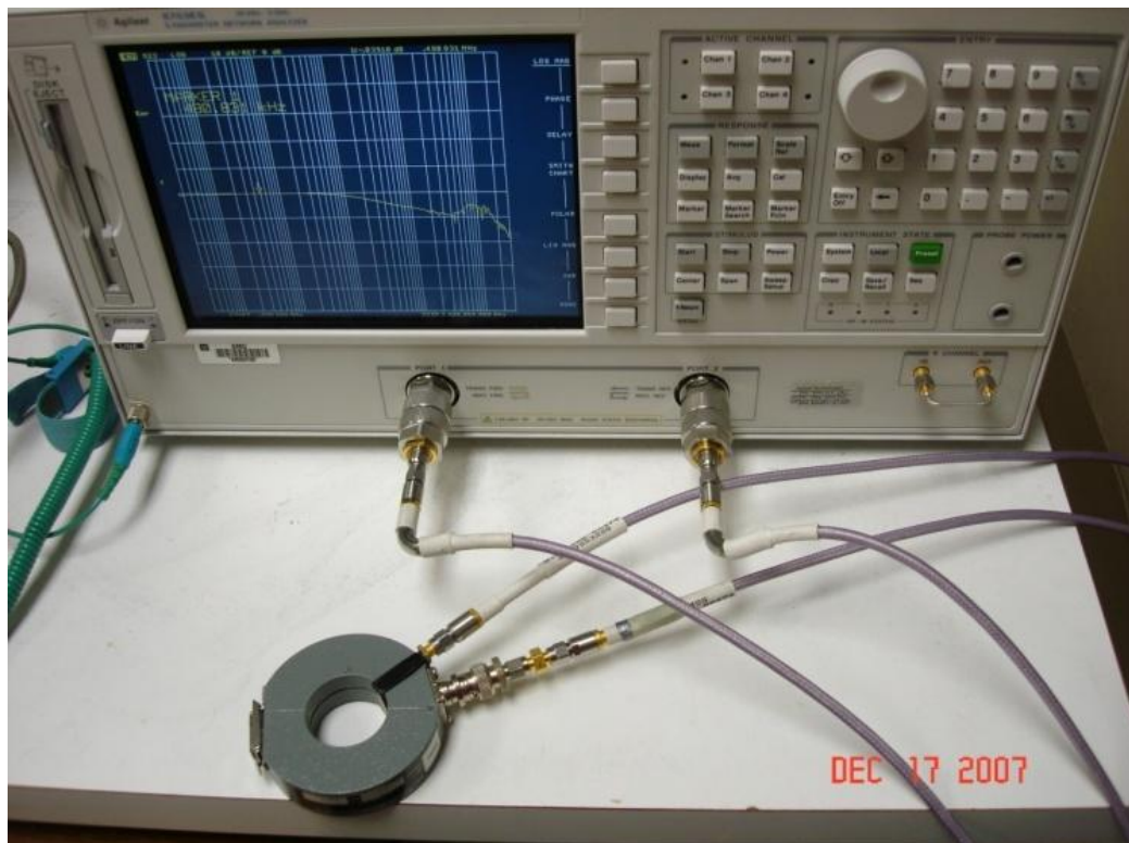
Figure 4.5. Current Probe Transfer Impedance Measurement Setup
