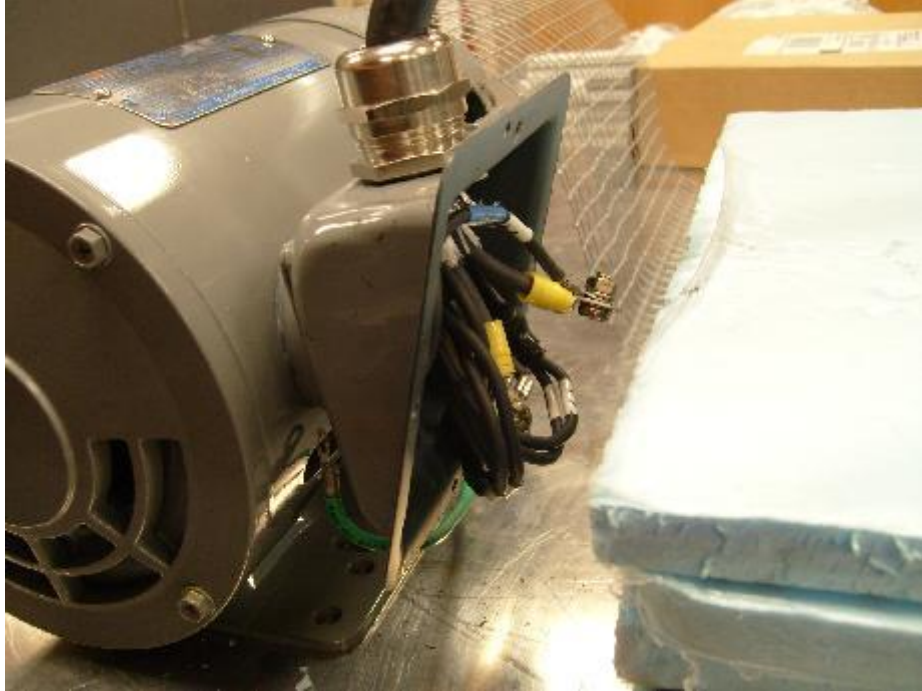
Figure 28 - Shielded Motor and Cable Test Setup: Motor Wiring
