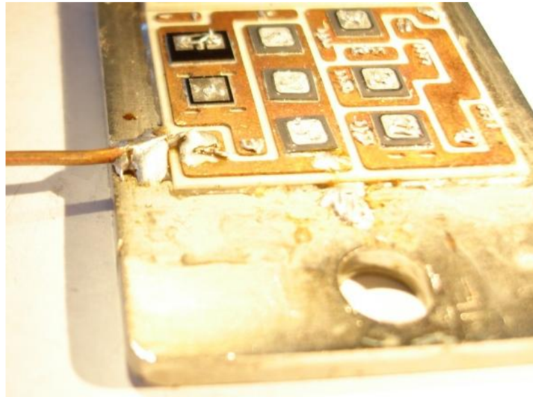
Figure 2.22. Measurement Setup for Area Fill B Capacitance
