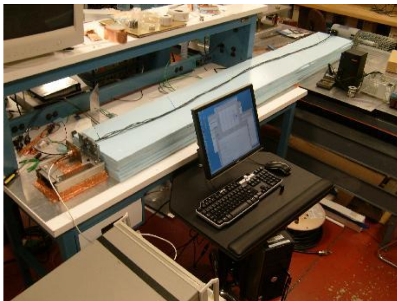
Figure 30 - Unshielded Motor and Cables Ground Wire Study Setup: Full View
