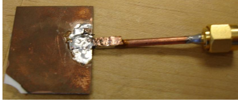
Figure 2.18. Substrate Capacitance Measurement Setup for Outer Conductor Connection
