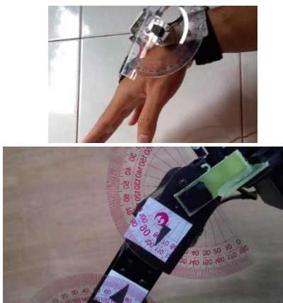
Figure 8: Measurement the arm angle and the robotic angle
