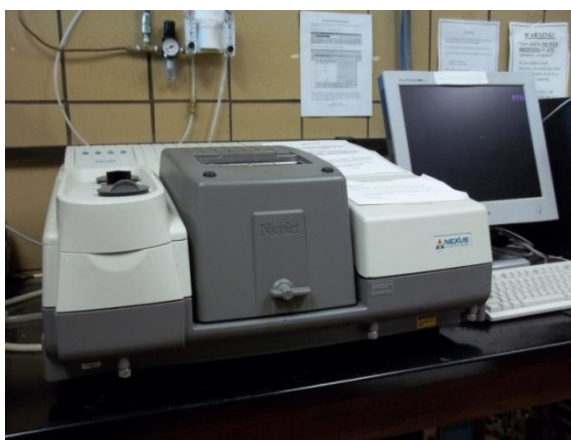
Figure 4.4. FTIR spectrometer NICOLET NEXUS 470.
