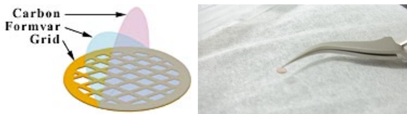
Figure 4.6. Schematic steps for sample preparation for STEM/TEM.
