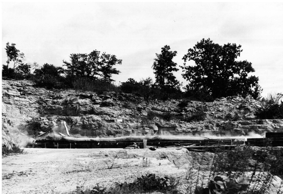
Figure 34. A \frac{1}{4} pound charge being detonated in Test Five, Phase II.
