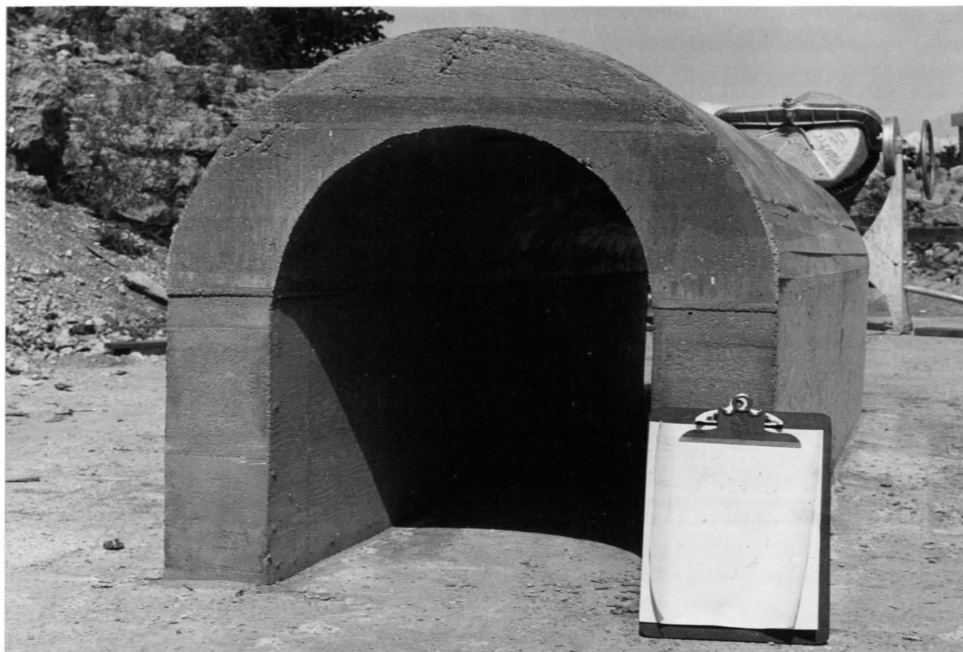
Figure 24. Type A tunnel constructed for Test Three, Phase One.
