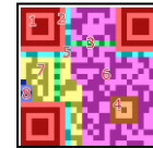
Figure 3: The structure of QR code version 2
