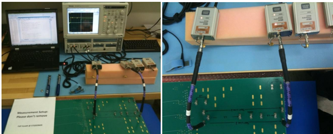
Figure 1.36: Measurement setup for the Tektronix DSA 8200
