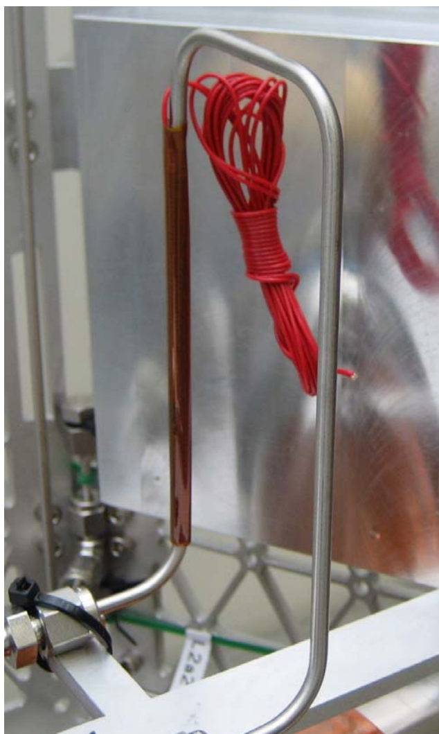
Figure 5.12 Heater Attached to Line
