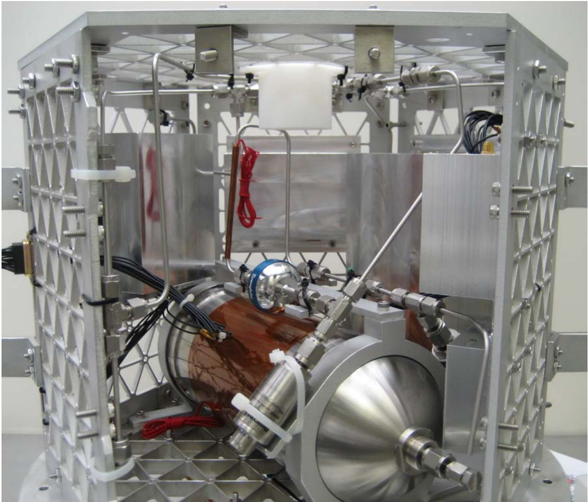
Figure 10.1 Propulsion System Integrated in MR SAT Structure
