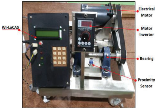
Figure 8: A Custom Made Testing Rig Using an Ac Motor for Proximity Sensor Performance Validation in Rotational Speed Measurement
