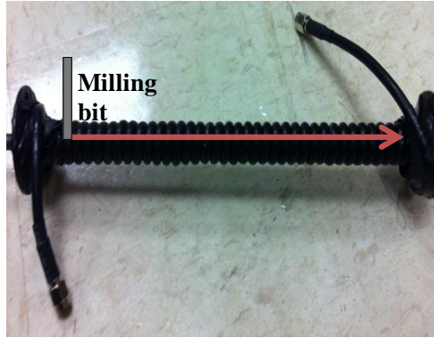
Figure 3.6. Image of a coiled coaxial cable resonator.
