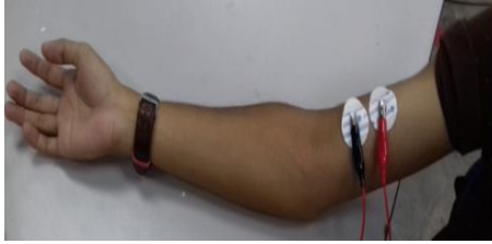
Figure 2: Electrodes placement on bicep muscle
