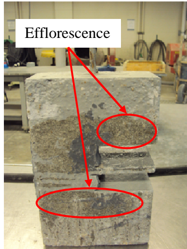
Figure 4.5. Efflorescence on specimen SP3-CI-10
