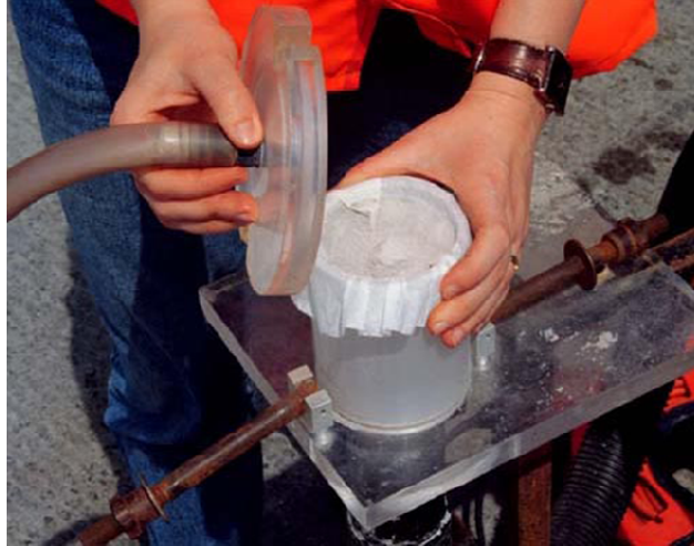
Figure 2.8. Powder concrete collection unit (Zemajtis 1998)
