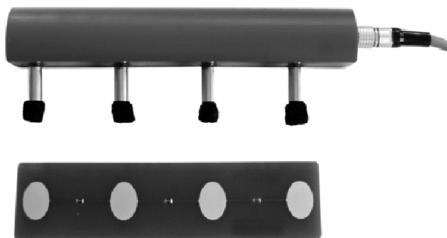
Figure 3.8. Electrical resistivity measurement (Proceq SA 2007)
