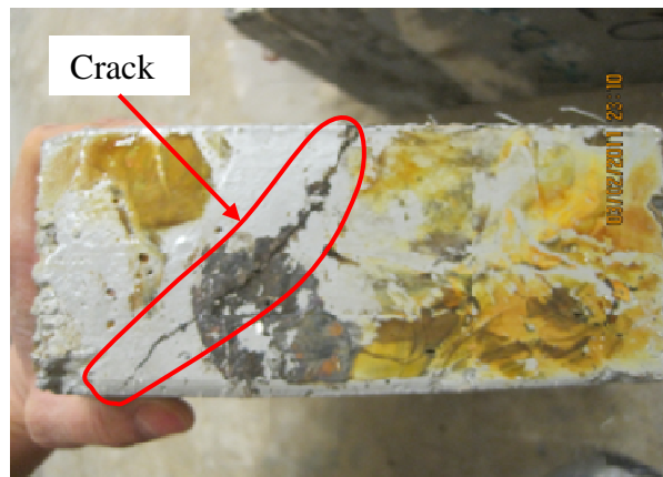
Figure 4.21. Cracks on specimen
