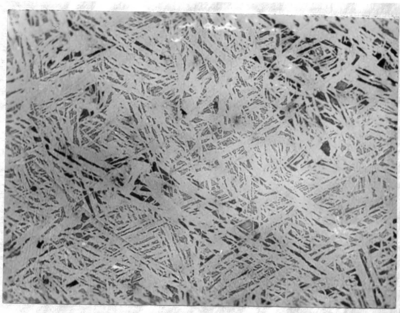
FIGURE 1A CAST STRUCTURE, NO. 6 HEAT 250x 3% NITAL ETCH 8 SECONDS
