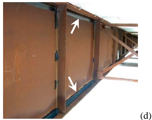
Figure 5 – Installation of optical fiber circuit: (a) schematic of sensor location; (b) cart on Girders 1 and 2, Span 2; (c) sensors on Girder 2; and (d) sensors on Girder 5.
