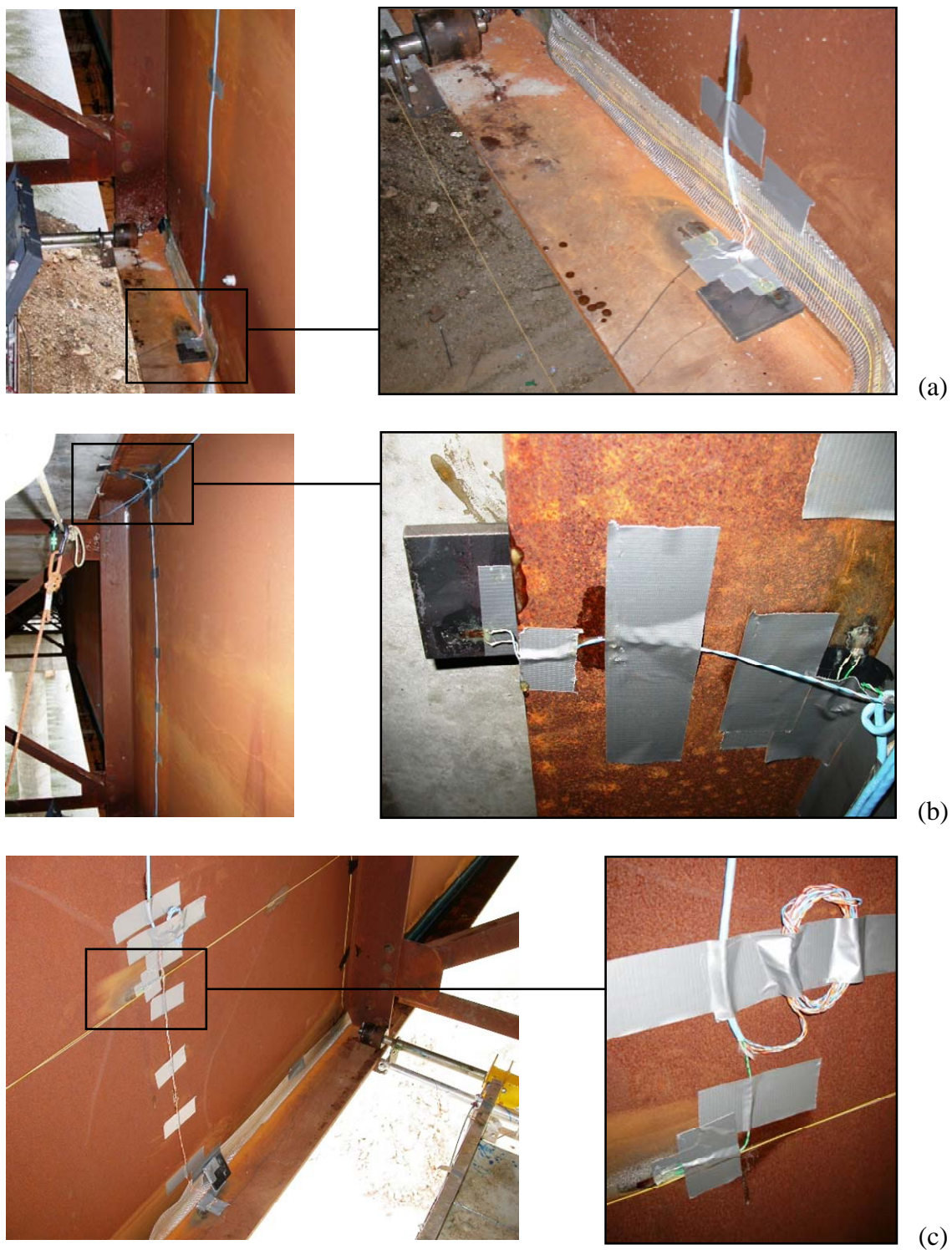
Figure 4 – Photographs of bonded and unbonded strain gauges on Girders 1 and 2: (a) Girder 1, bottom flange; (b) top flange; and (c) Girder 2, bottom flange and Location II.
