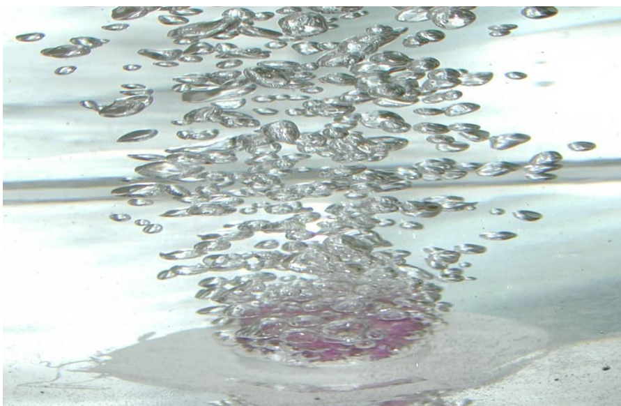
Figure 2.7. Argon Bubbles Rise from Core Drilled Porous Plug Being Tested in Water
