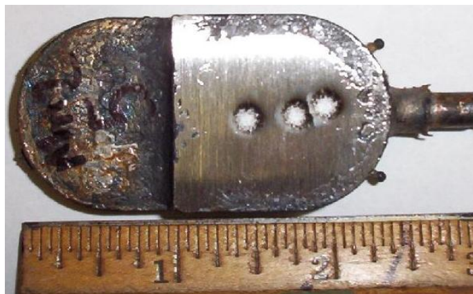
Figure 2.11. Photograph of a Steel Specimen Obtained from a Tundish Sampler after Sanding and Chemical Analysis Using an Arc-spectrometer (note: scale in inches)
