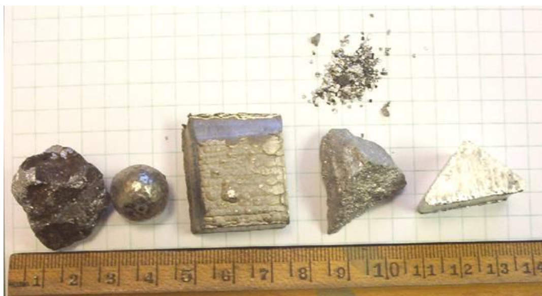
Figure 2.15. Photograph of Alloys Used to Study Dissolution. Left to Right: Low Carbon Ferromanganese Lump, Nickel Pellet, Nickel Cathode, Ferroniobium (granular above lump), Tin Cut from Triangular Bar (note: scale in centimeters)
