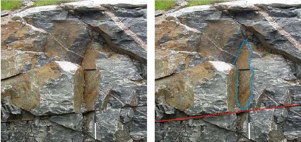
Figure 1.6. A rock cut containing both fracture traces (red line) and facets (cyan polygon) (Otoo et al., 2011)
