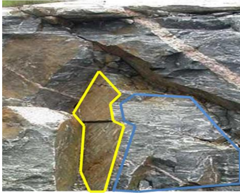
Figure 4.4. Rock face showing both a relatively smooth, stained, natural facet (yellow polygon) and an induced facet (blue polygon).
