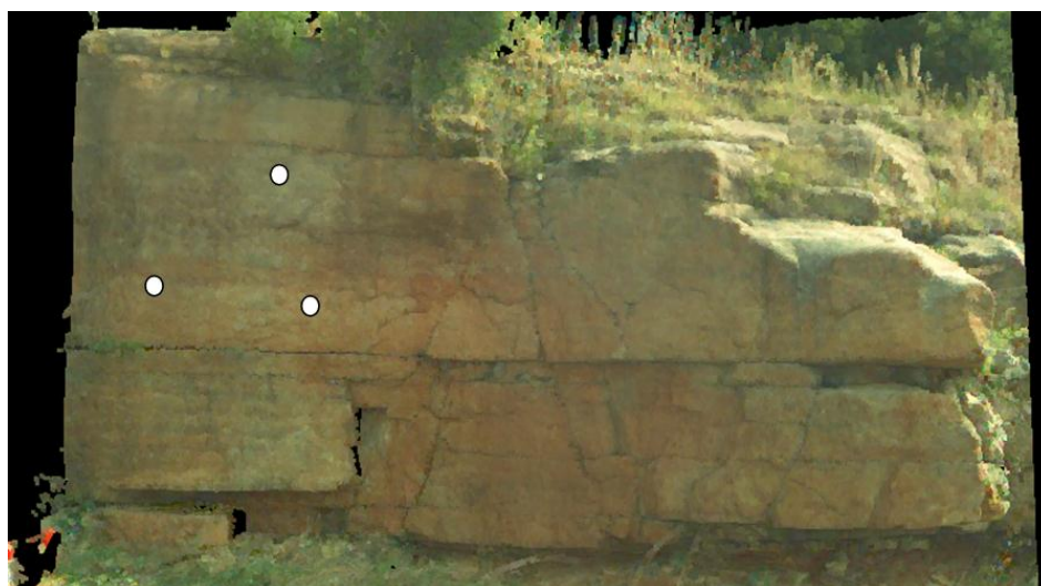
Figure A.1. 3 selected points on a rock face. The azimuth of the portion of the rock face with the 3 points represents the azimuth of the rock face.
