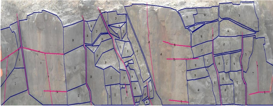
Figure 3.13. Manually prepared facet and trace map of a rock face in Rolla, Missouri. Red lines represent linear traces and blue polygons represent planar facets.
