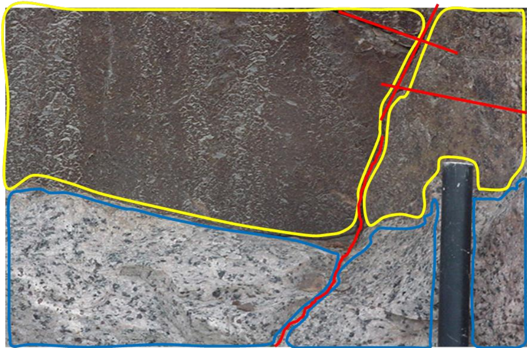
Figure 1.7. Image of a rock cut showing natural facets (joint surface, yellow polygons), joint traces (red lines) and induced facets (blasted surface, blue polygons).
