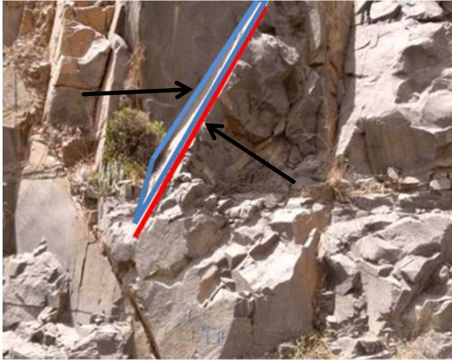
Figure 4.2. A rock cut showing a discontinuity occurring as a trace (red line) from one direction and a facet (blue polygon) from another direction.
