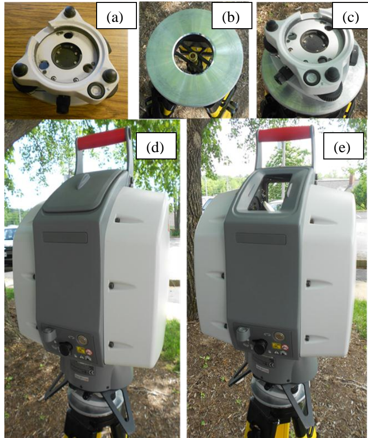
Figure 3.9. (a) Tribrach, with its optical plummet pointing to the front, (b) Head of tripod, with the screw for mounting the tribrach, (c) Tribrach mounted on tripod, (d) Scanner mounted on tribrach and tripod, leveled and locked in place with windows closed (e) Scanner mounted on tribrach and tripod, leveled and locked in place with windows opened.
