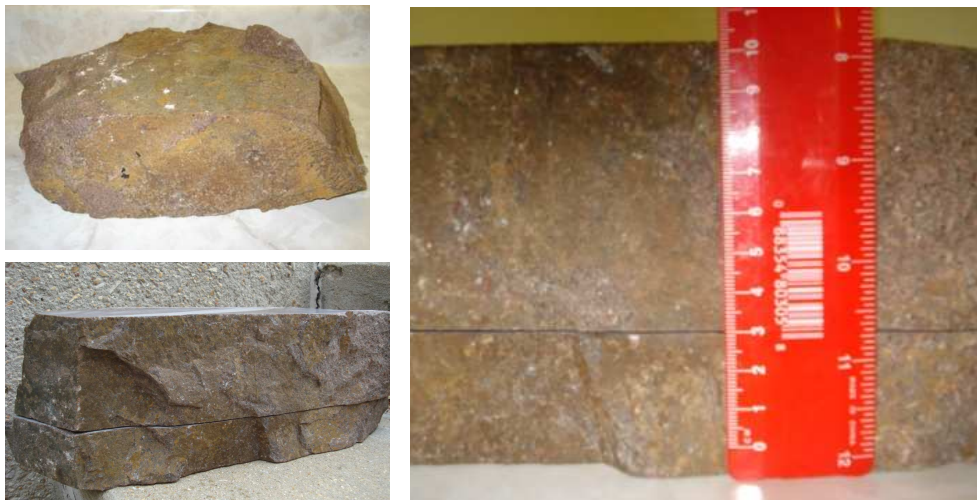
Figure 5.9: The ignimbrite rock sample from Madison County-MO and the trimmed two blocks of the sample in order to conduct a lab measurement for the velocity of the GPR pulses that travel through this type of igneous rock. The Thickness of the top block is 7.40 cm.
