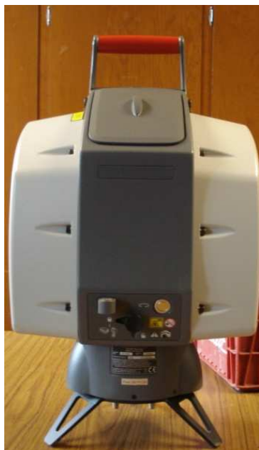
Figure 5.30: A Leica ScanStation II (LIDAR scanner) which was used in this study.
