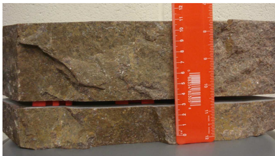
Figure 5.11: The two blocks of ignimbrite rock sample were positioned on top of each other to create an artificial joint with a filled-air aperture of 0.8 cm wide.
