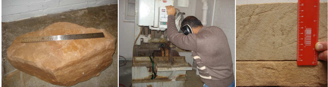
Figure 5.8: The sandstone sample from Phelps County-MO and the trimmed two blocks of the sample in order to conduct a lab measurement for the velocity of the GPR pulses that travel through this type of sedimentary rock. The thickness of the top block is 10.60 cm.
