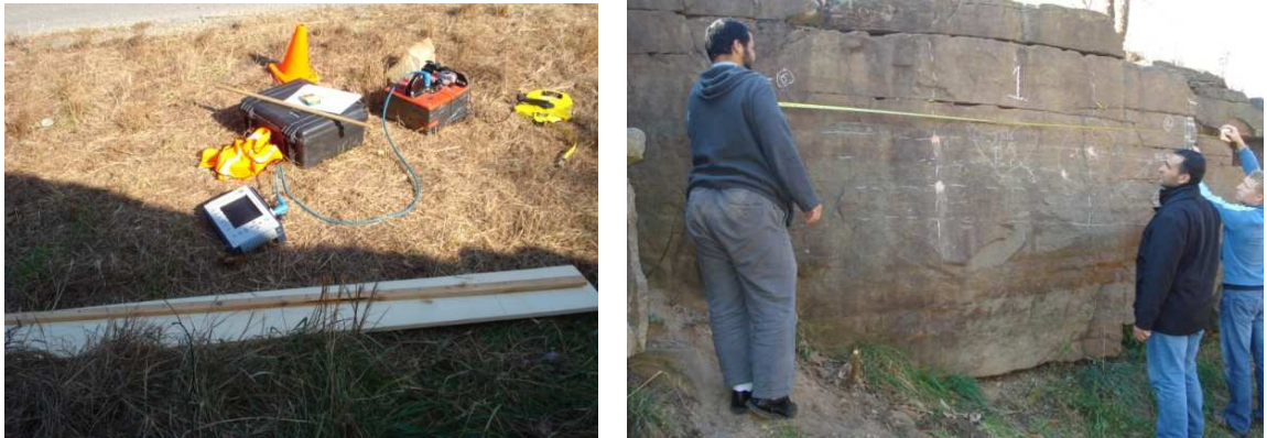
Figure 5.25: A wooden panel was used as a try to create a smooth surface on which the GPR antenna was towed at St.1 (left image), while the right image shows the process of drawing using chalk the location of the GPR survey lines on the rock slope face.
