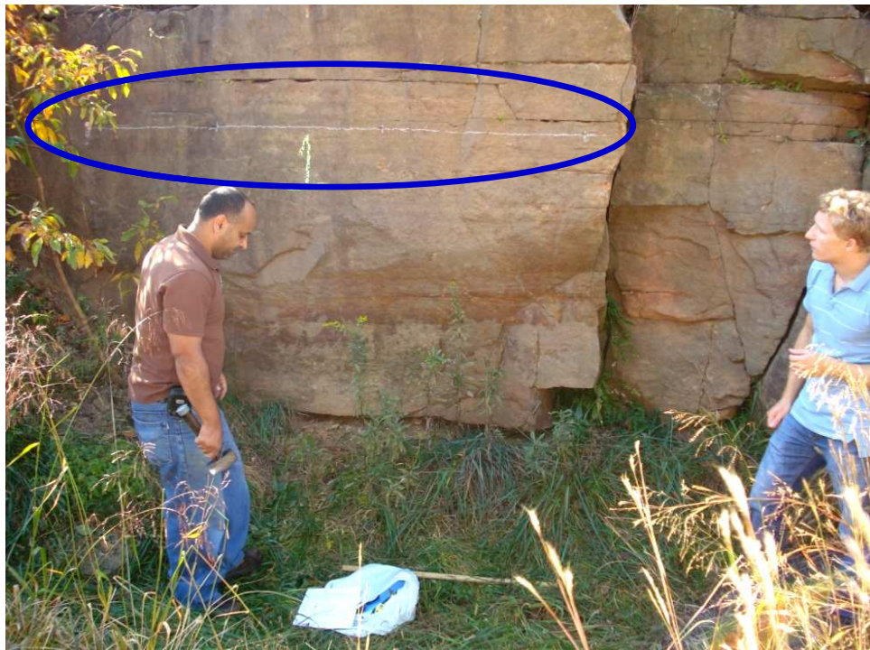
Figure 5.4: Shows the location (blue circle) of where the tape measurement should be for scanline survey at St.1. Notice that the scanline did not intersect with more than three joints on the rock face which push us to measure manually the orientation of all accessible joints without relying on the scanline itself.
