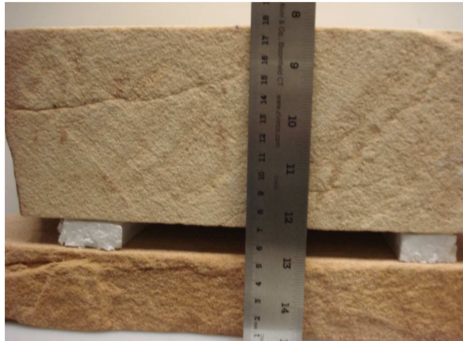
Figure 5.10: The two blocks of sandstone rock sample were positioned on top of each other to create an artificial joint with a filled-air aperture of 1.8 cm wide.
