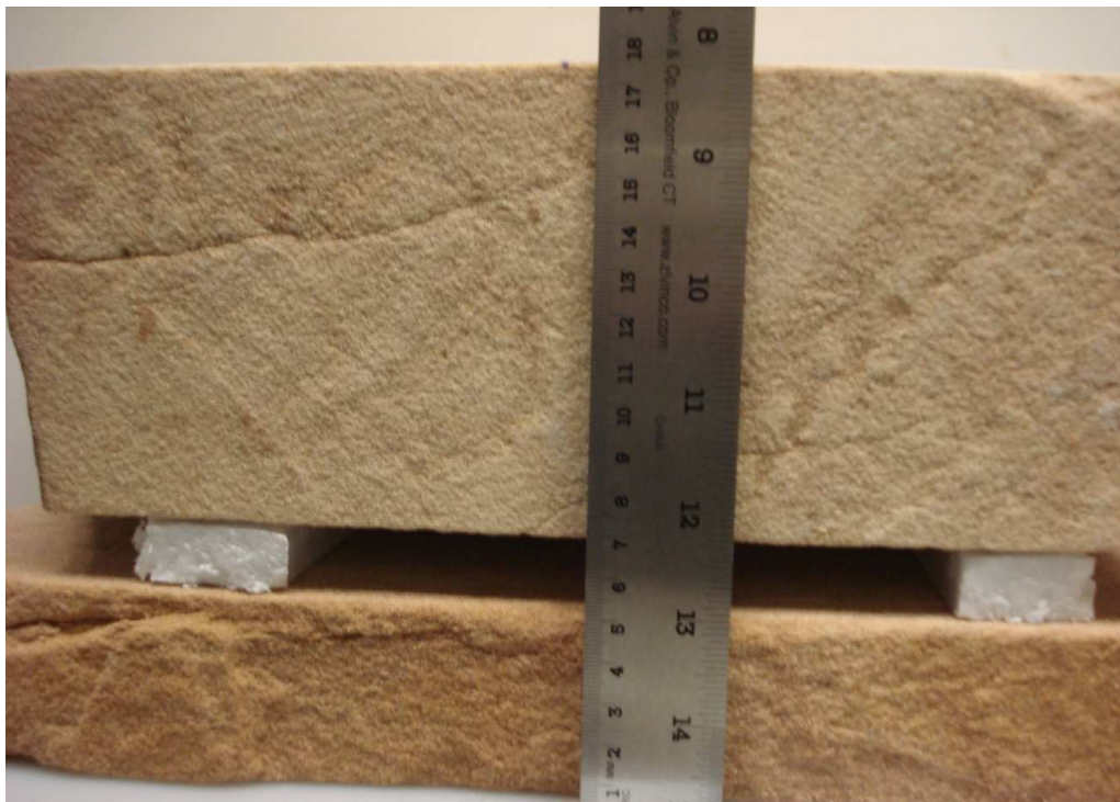
Figure 5.12: The thickness of the top block is 10.50 cm which means the true perpendicular (vertical) depth to the created discontinuity is 10.50 cm. The separation between the two blocks was 1.80 cm.
