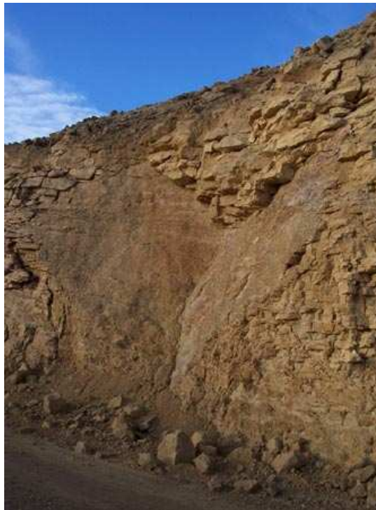
Figure 2.10: A wedge failure along two intersecting planes of discontinuities both of which daylight in the slope face in a limestone quarry (Adopted from http://www.bgs.ac.uk/eqr/SlopeStability.htm ).
