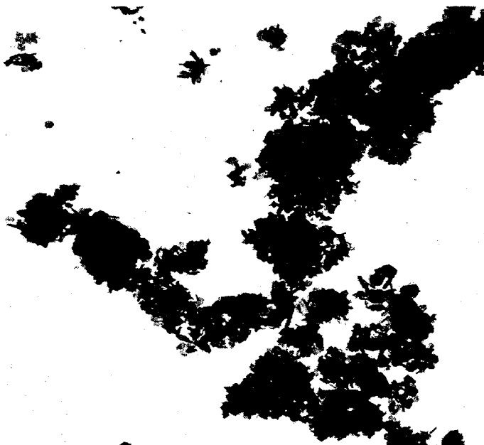
Figure 30. Electron Micrograph of Sample Calcined 8 Hours at 900°C (10,000X)
