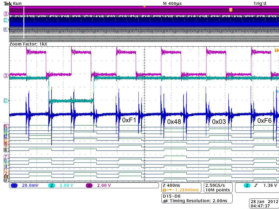
Figure 3.5. Power waveform of NCL S-Box design.
