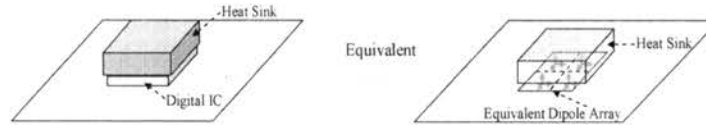
Fig. 2. Generating a realistic excitation for heat-sink studies using dipole moments to replace the IC underneath the heat sink.
