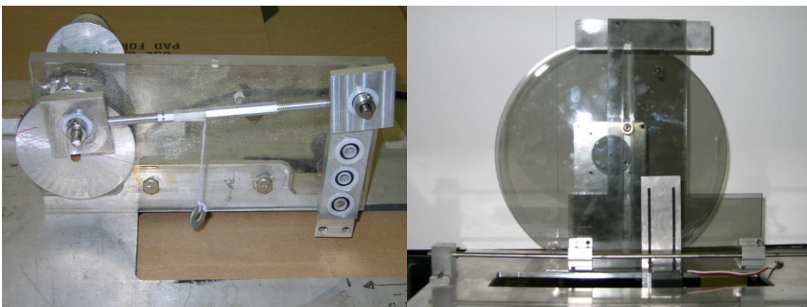
Figure 3-2: Flapping (left) and plunging (right) mechanisms.
