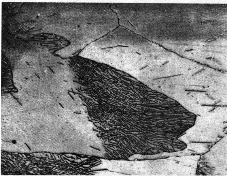
Figure 3. Zn-2at.%Cu, solution treated 12 hours at 400°C, aged 36 hours at 200°C. X200 (54)
