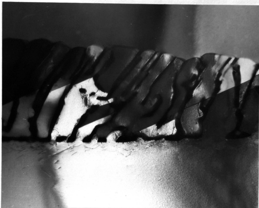
Figure 22. Cu-9.5at.%In, solution treated 5 minutes at 625°C, water quenched and aged 15 minutes at 428°C. Cellular precipitate. X14,400
