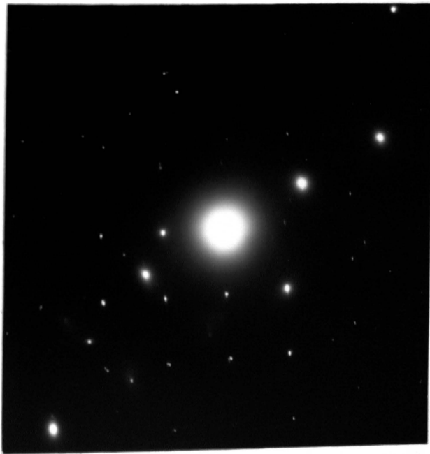
Figure 54b. Selected area diffraction pattern of the cellular lamellae in Figure 54a. Rotated 44° counterclockwise from Figure 54a. \lambda = 3.47 \text{ \AA} .
