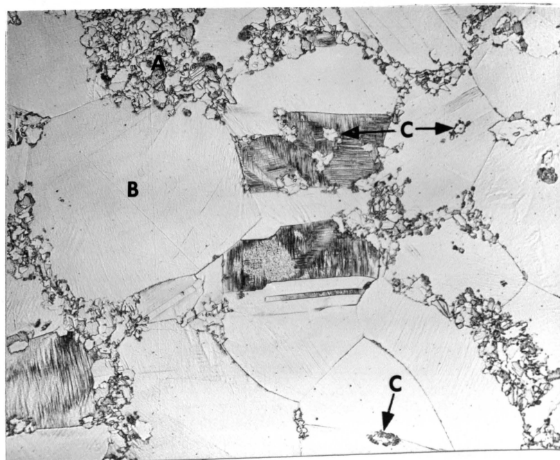
Figure 45. Cu-9.5at.%In, solution treated and water quenched, cold rolled 27%, solution treated 10 seconds at 625°C, isothermally aged 15 minutes at 420°C. A partially recrystallized and aged structure. X75
