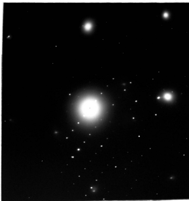
Figure 55b. Selected area diffraction pattern of the cellular lamellae in Figure 55a. Rotated 26° counterclockwise from Figure 55a. \lambda=3.54\text{\AA} .
