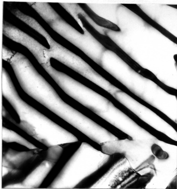
Figure 54a. Cu-9.5at.%In, solution treated 5 minutes at 623°C, water quenched, aged 30 minutes at 428°C. Cellular lamellae. X32,500
