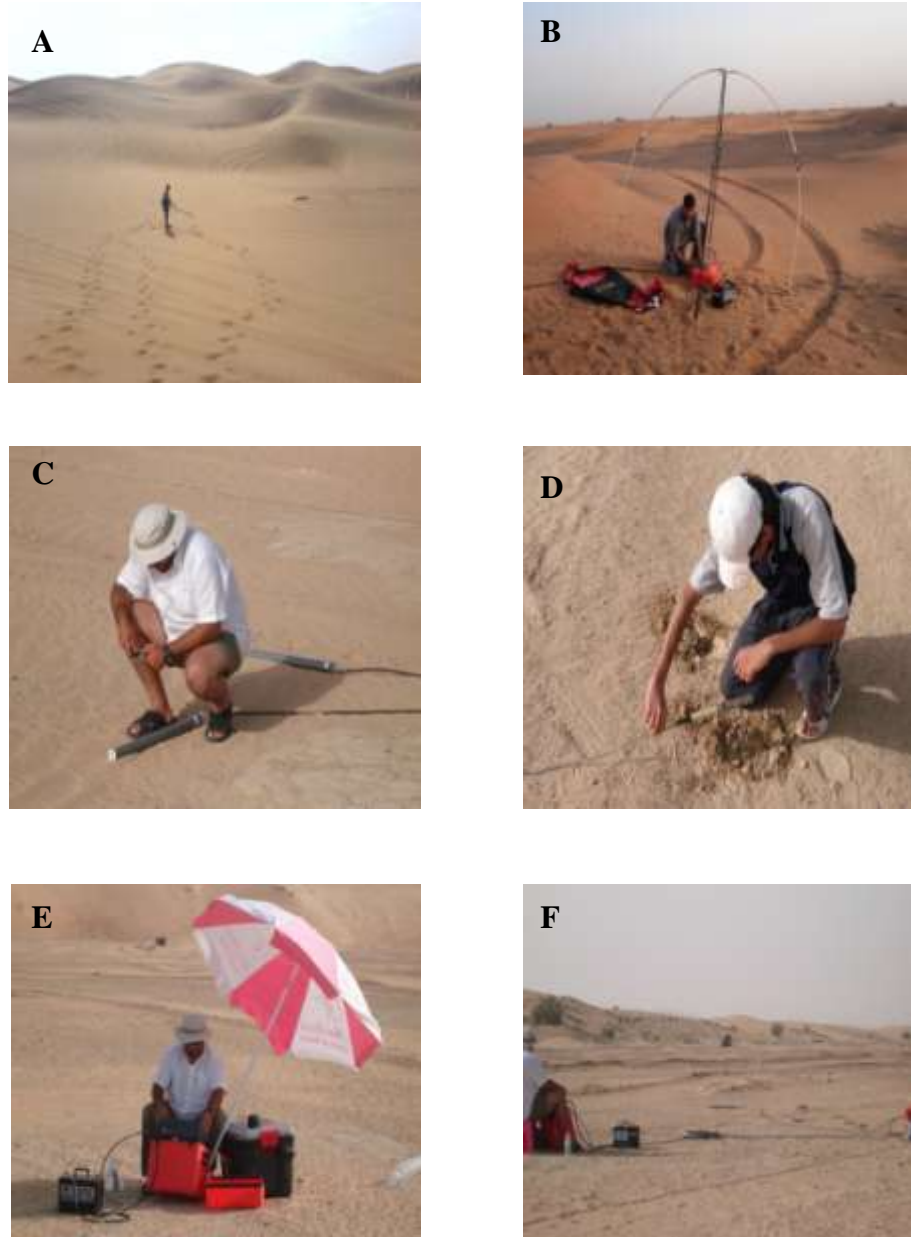
Figure A.8 Images of the field work, A) Magnetic survey, B) Transmitter (CSAMT Survey) C) Magnetometer coil (CSAMT Survey) D) Electrode (CSAMT Survey) E) Operating console (CSAMT) F) General layout during the operation.
